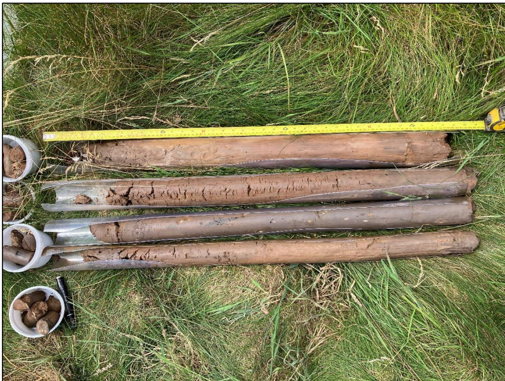
Photograph 39 – Photograph of the Hummocky Glacial Deposits between 1.2 – 5.0m depth bgl in WS03.
