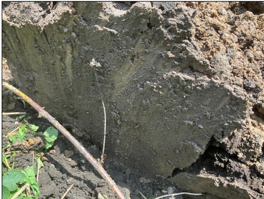
Photograph 59 – Photograph of Hummocky Glacial Deposits encountered in TP20.
