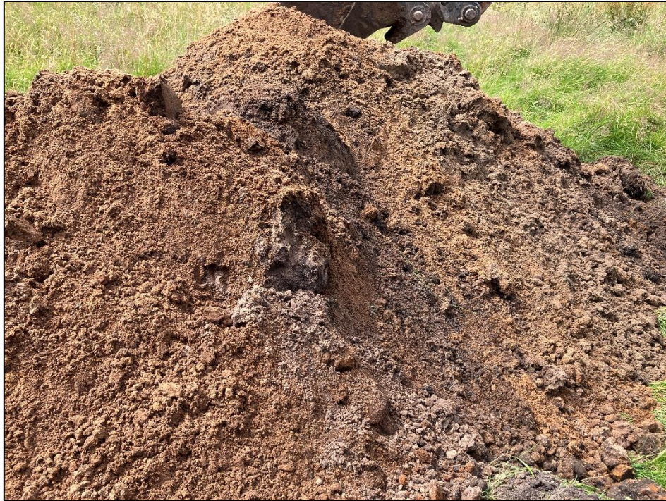
Photograph 62 – Photograph of the Hummocky Glacial Deposits encountered in TP21.
