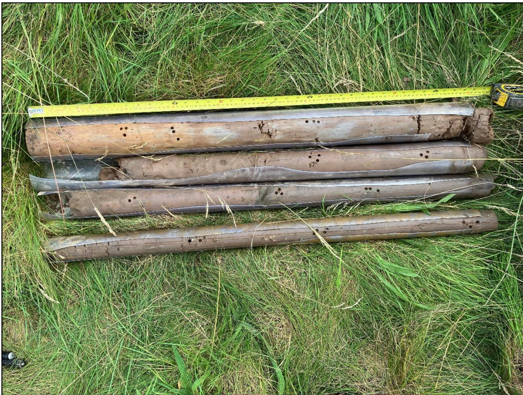
Photograph 37 – Photograph of the Hummocky Glacial Deposits between 1.2 – 5.0m depth bgl in WS02.
