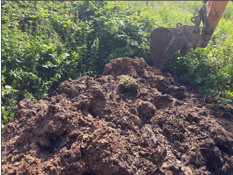
Photograph 58 – Photograph of Made Ground encountered in TP20.
