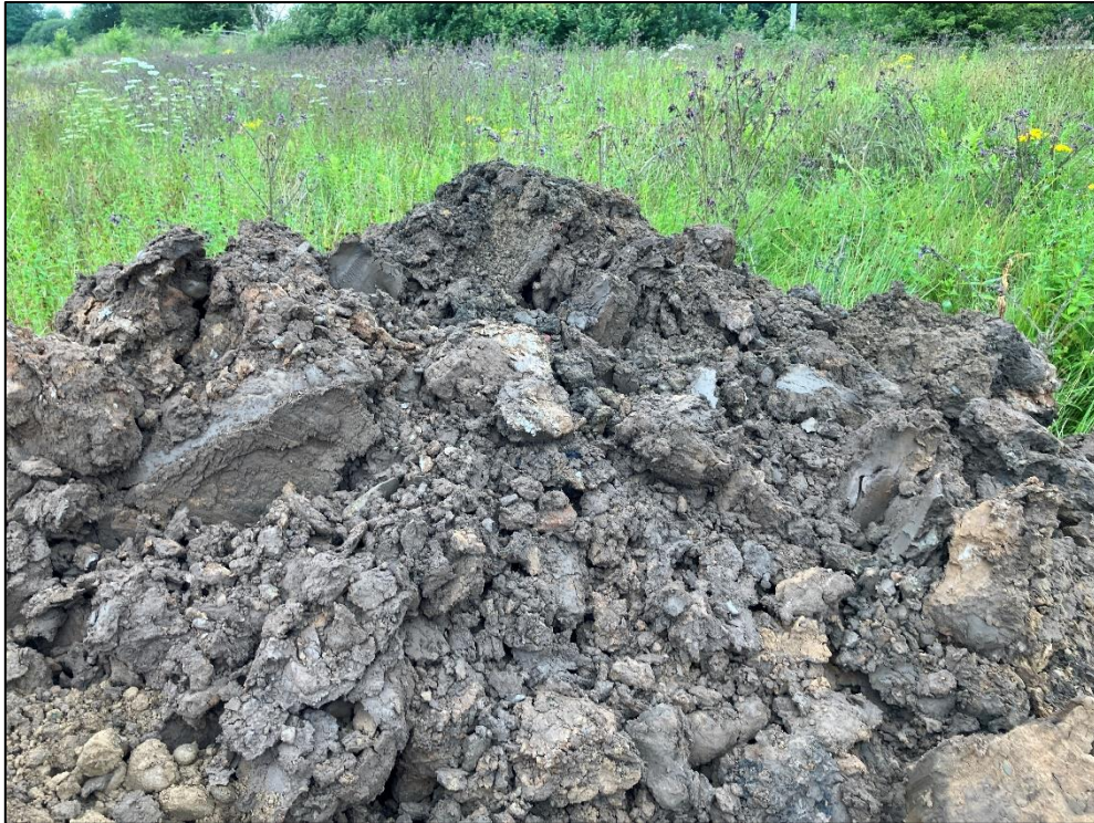
Photograph 21 – Photograph of the Hummocky Glacial Deposits encountered in TP07.
