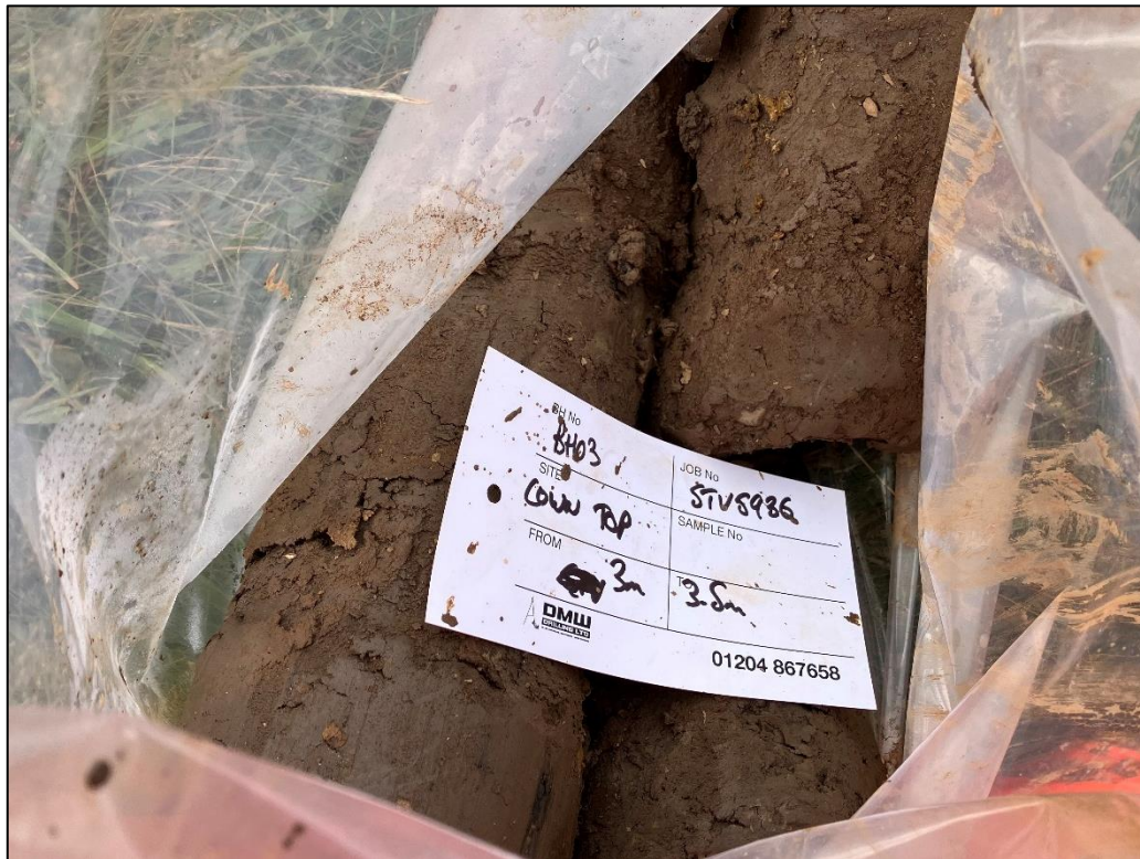
Photograph 9 – Photograph of the Hummocky Glacial Deposits between 3.0 – 3.5m bgl in BH03.
