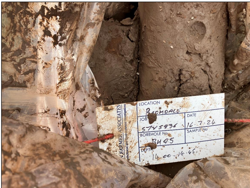
Photograph 16 – Photograph of the Hummocky Glacial Deposits between 14.0 – 14.45m depth bgl in BH05.
