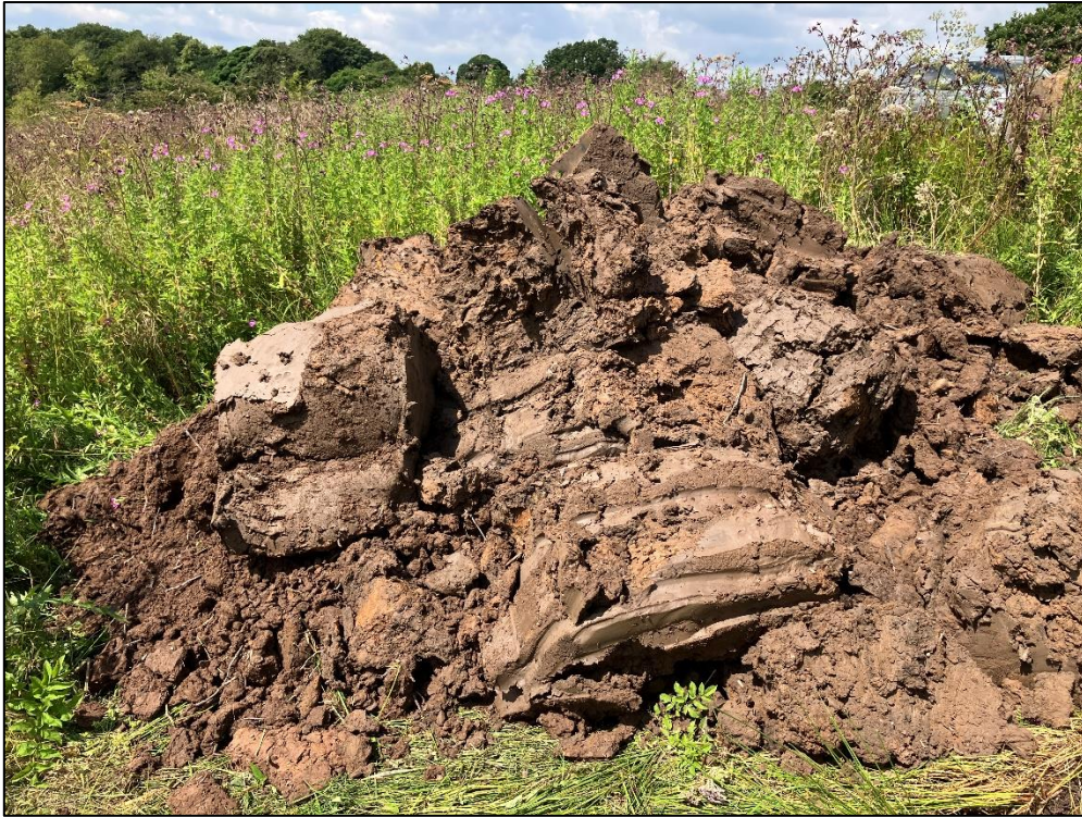
Photograph 40 – Photograph of the Hummocky Glacial Deposits encountered in TP13.
