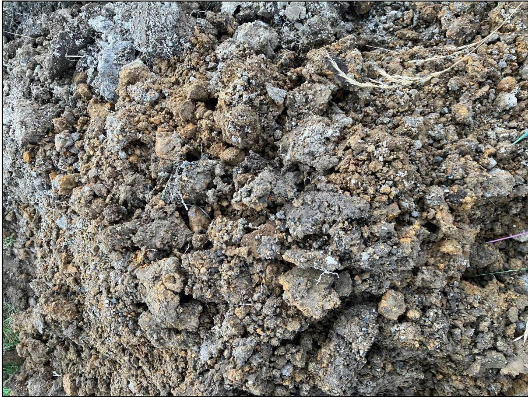
Photograph 36 – Photograph of the Hummocky Glacial Deposits between 0.4 – 1.2m depth bgl in WS02.
