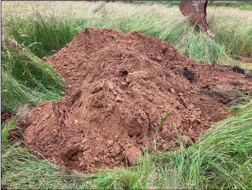
Photograph 3 – Photograph of the Hummocky Glacial Deposits encountered in TP01.
