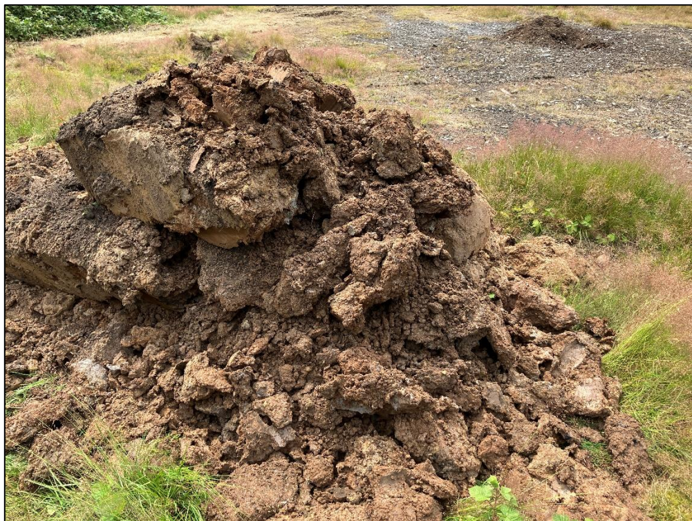
Photograph 71 – Photograph of Hummocky Glacial Deposits encountered in TP26.
