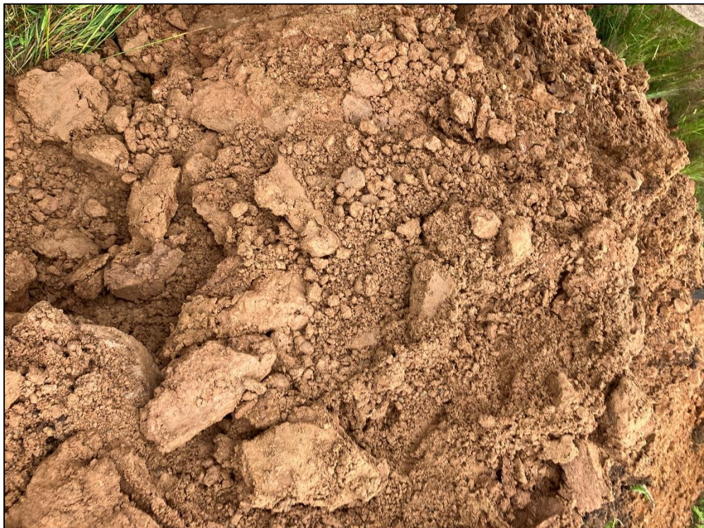
Photograph 6 – Photograph of the Hummocky Glacial Deposits encountered in TP02.
