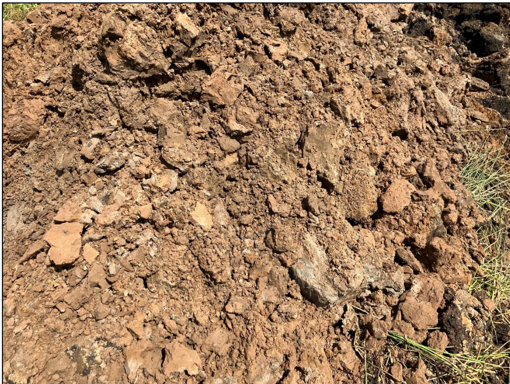
Photograph 24 – Photograph of the Hummocky Glacial Deposits encountered in TP08.
