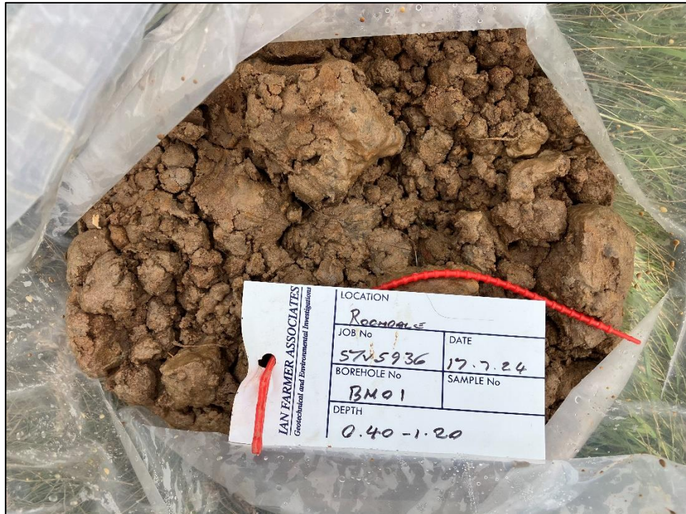
Photograph 1 – Photograph of the Hummocky Glacial Deposits between 0.4-1.2m bgl in BH01.
