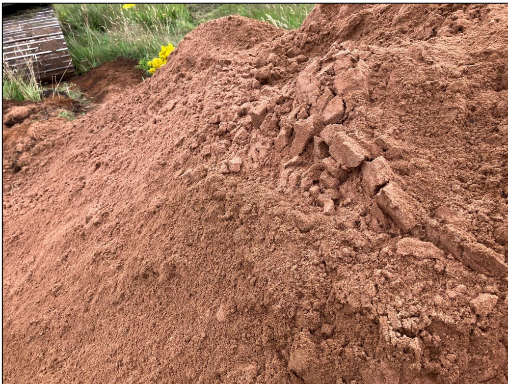
Photograph 65 – Photograph of the Hummocky Glacial Deposits encountered in TP22
