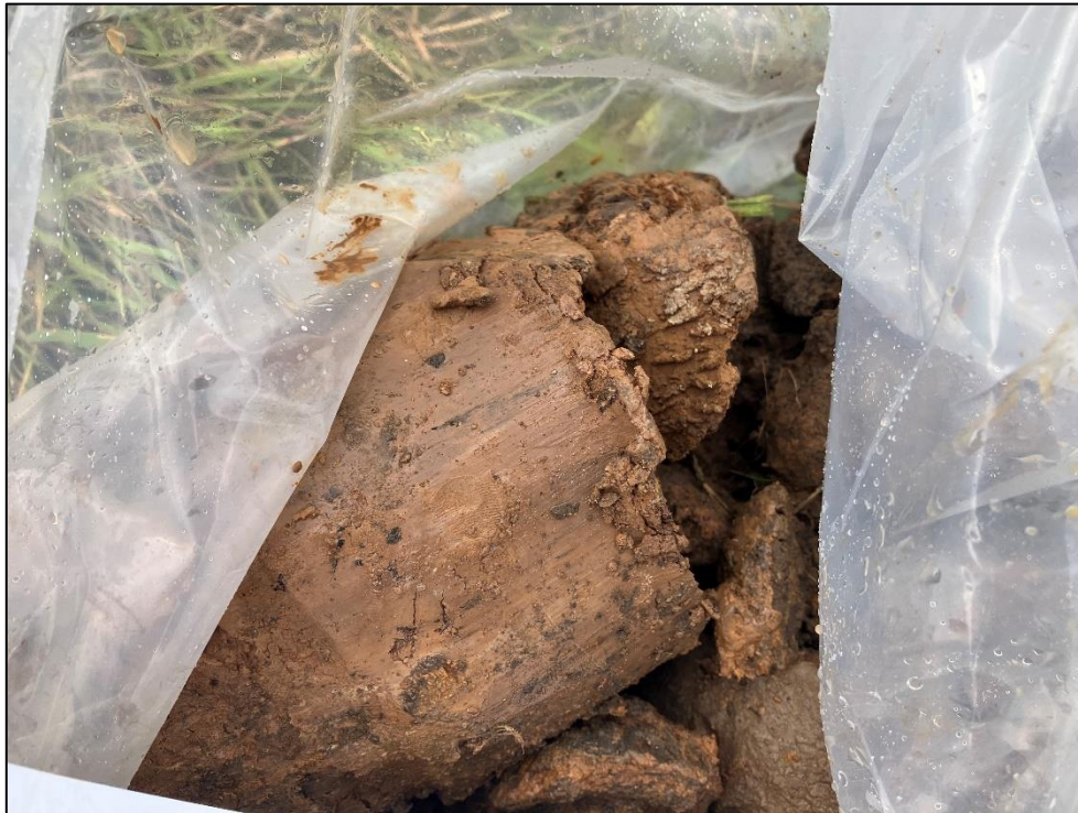
Photograph 5 – Photograph of the Hummocky Glacial Deposits between 0.40m and 1.00m in BH02.
