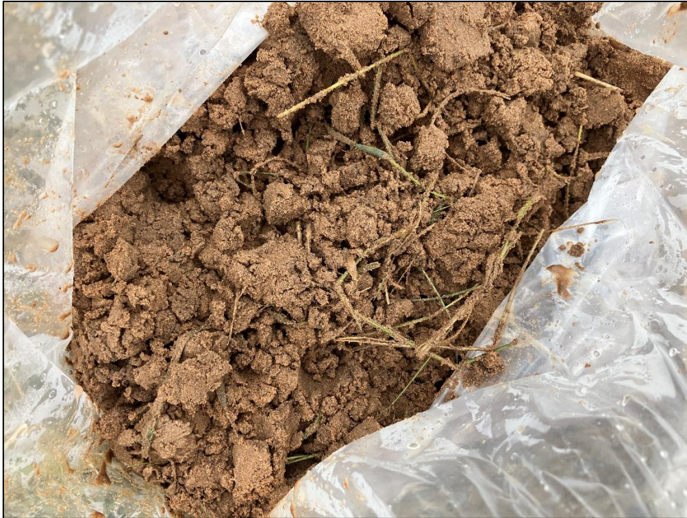
Photograph 23 – Photograph of the Hummocky Glacial Deposits between 8.0 – 8.45m depth bgl in BH08.
