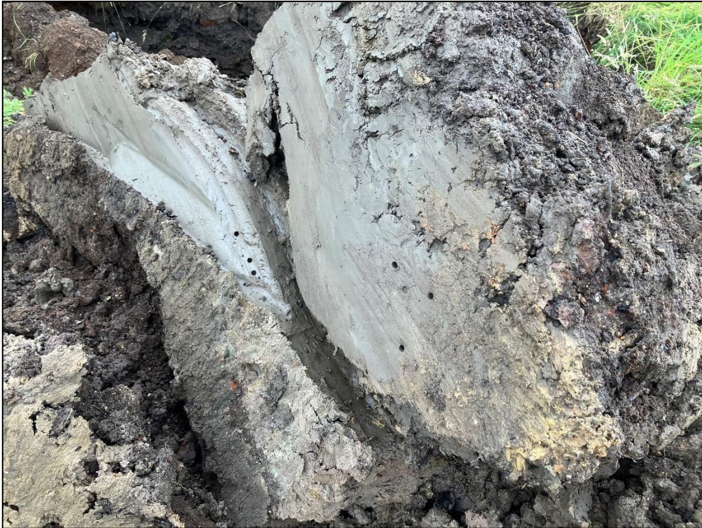
Photograph 9 – Photograph of the Hummocky Glacial Deposits encountered in TP03.
