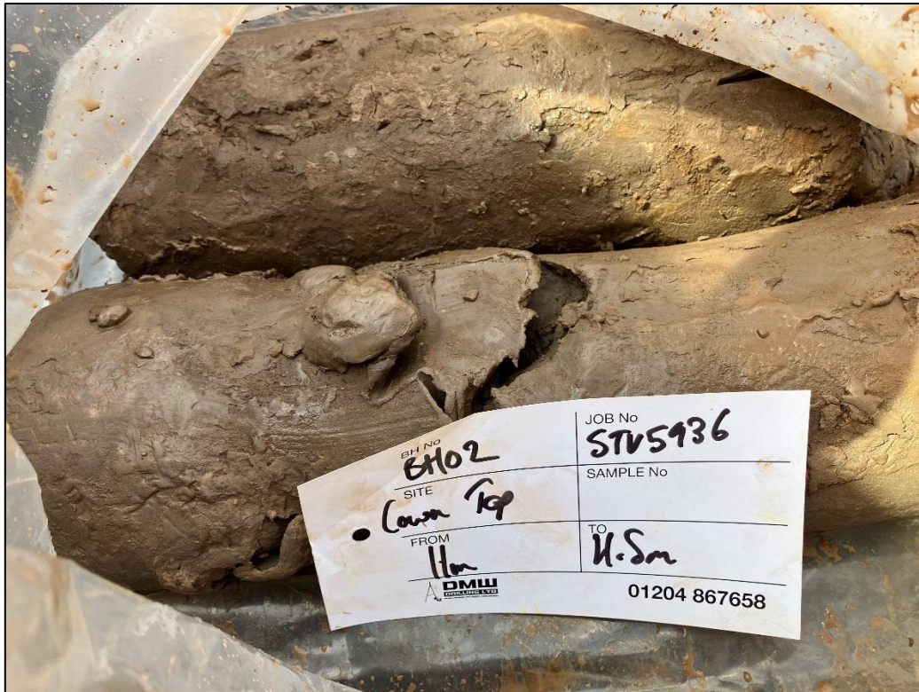
Photograph 7 – Photograph of Hummocky Glacial Deposits between 11.0 and 11.5m bgl in BH02.
