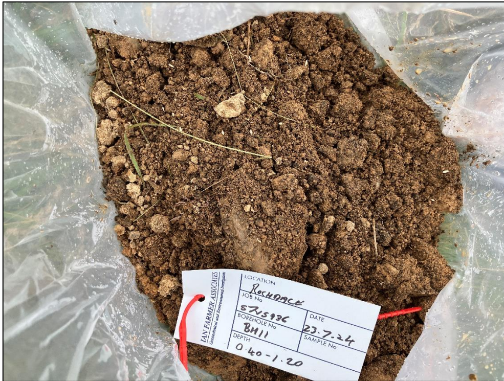
Photograph 29 – Phgotograph of the Hummocky Glacial Deposits between 0.4 – 1.2m depth bgl in BH11.
