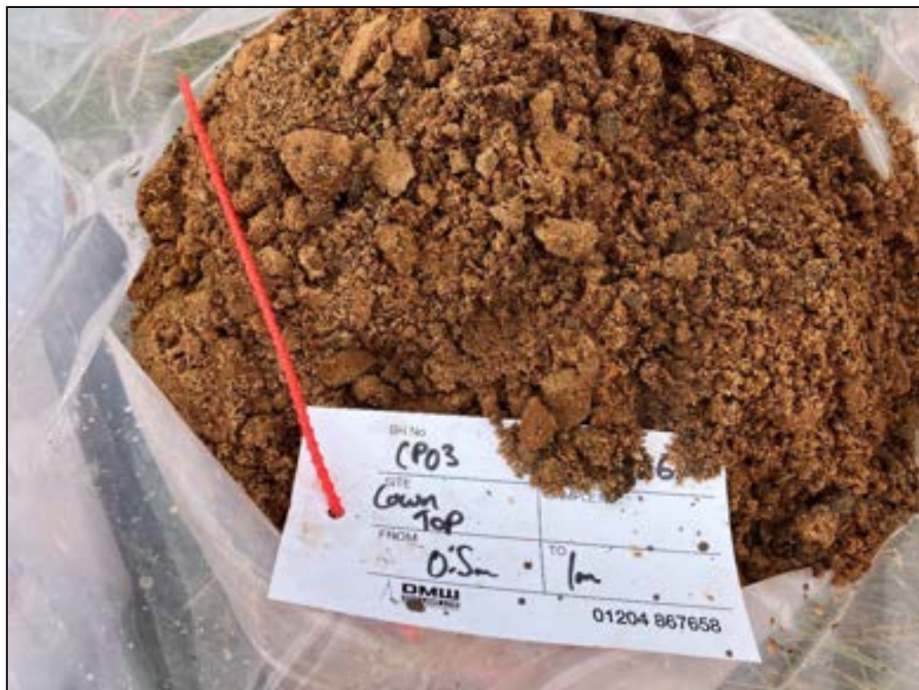
Photograph 8 – Photograph of the Hummocky Glacial Deposits between 0.50 – 1.0m in BH03.
