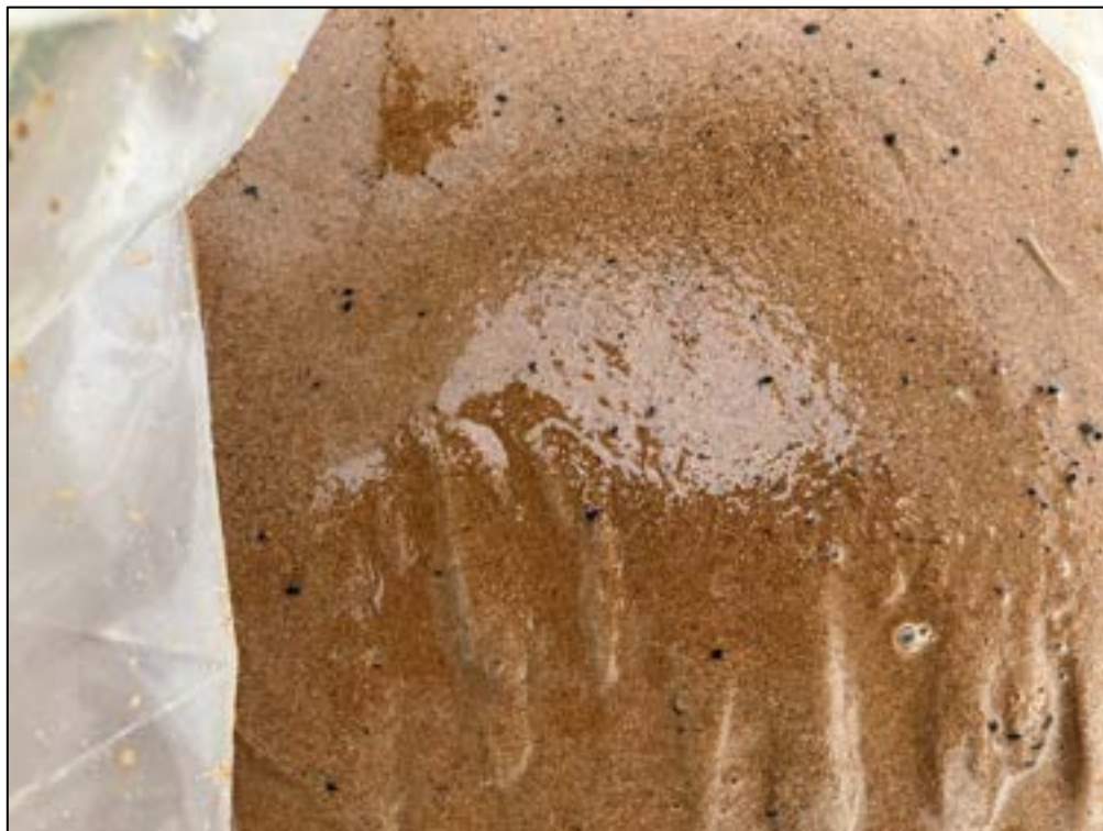
Photograph 24 – Photograph of the Hummocky Glacial Deposits between 13.5 – 13.95m depth bgl on BH08.
