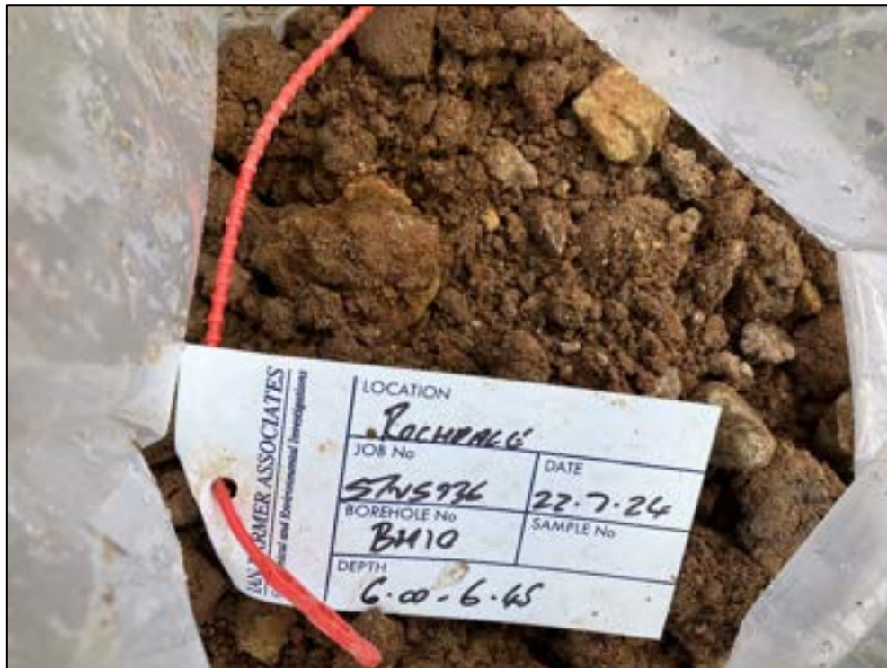
Photograph 28 – Photograph of the Hummocky Glacial Deposits between 6.0 – 6.45m depth bgl in BH10.
