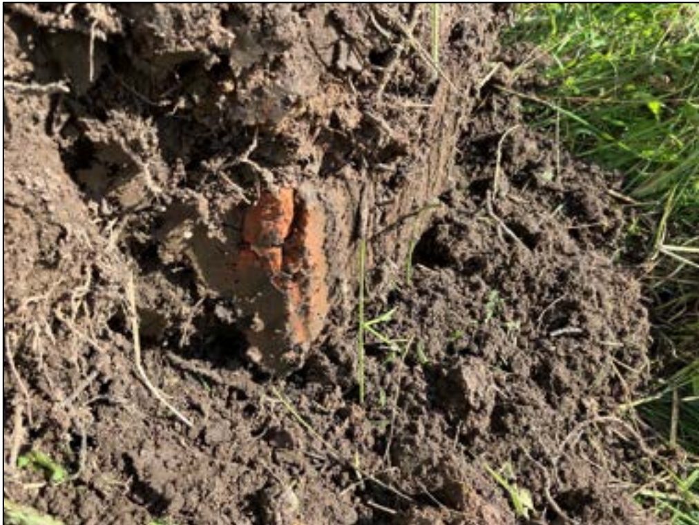
Photograph 39 – Photograph of the Made Ground encountered in TP13.
