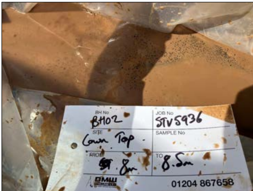
Photograph 6 – Photograph from the Hummocky Glacial Deposits between 8.0 – 8.5m in BH02.
