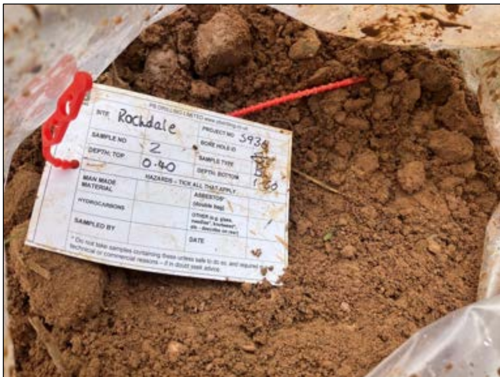
Photograph 22 – Photograph of the Hummocky Glacial Deposits between 0.40m and 1.2m depth bgl in BH08.
