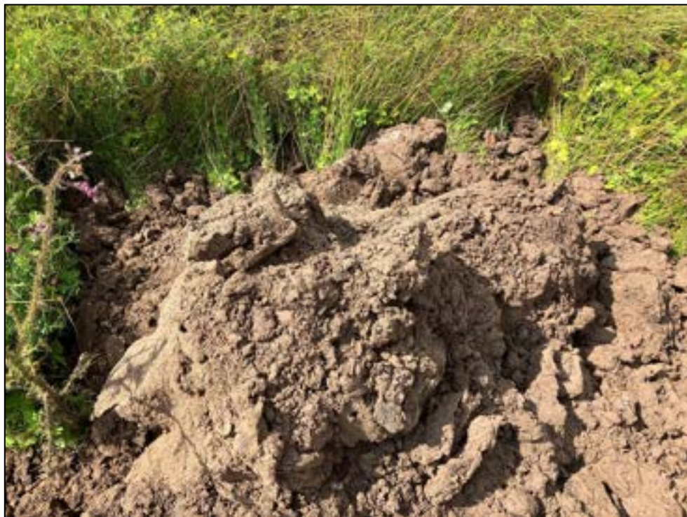
Photograph 33 – Photograph of the Hummocky Glacial Deposits encountered in TP11.
