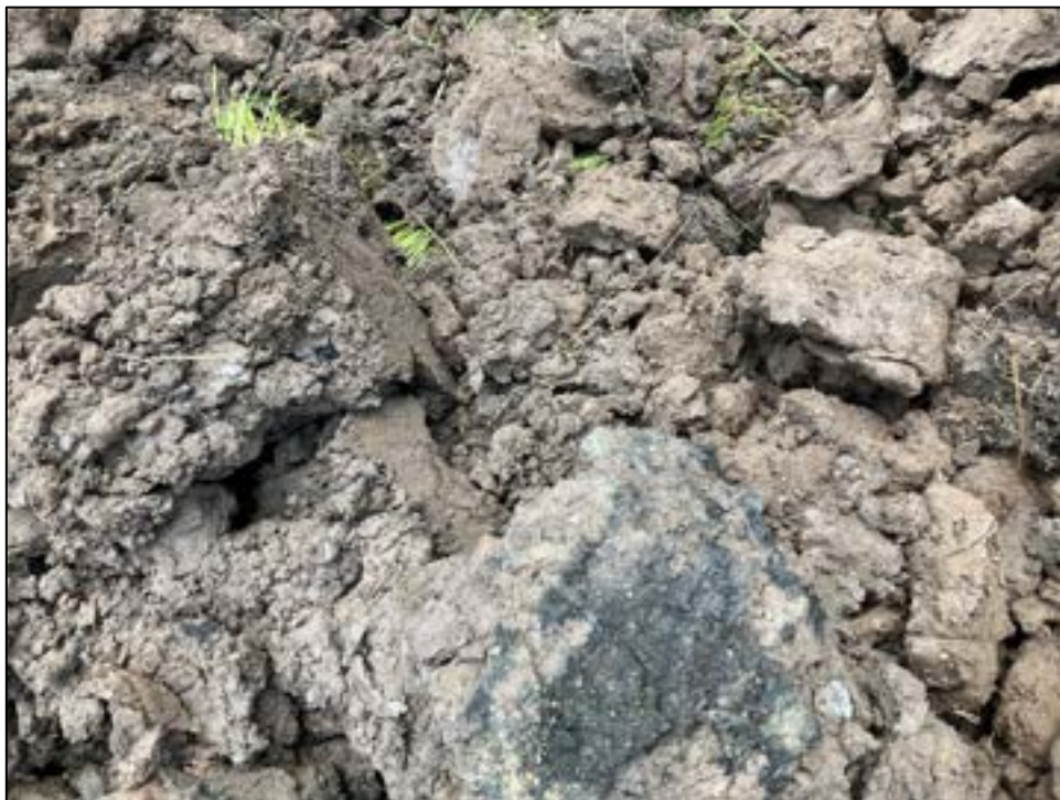
Photograph 43 – Photograph of the Hummocky Glacial Deposits encountered in TP14.
