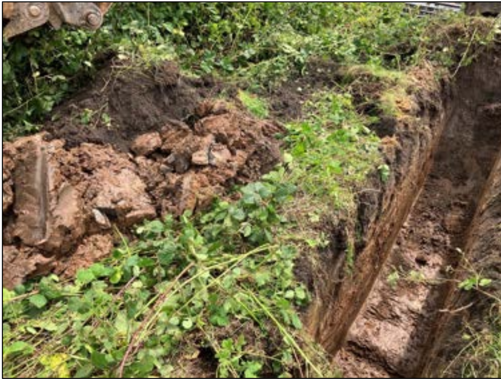
Photograph 70 – Photograph of TP26, with Topsoil pictured left.
