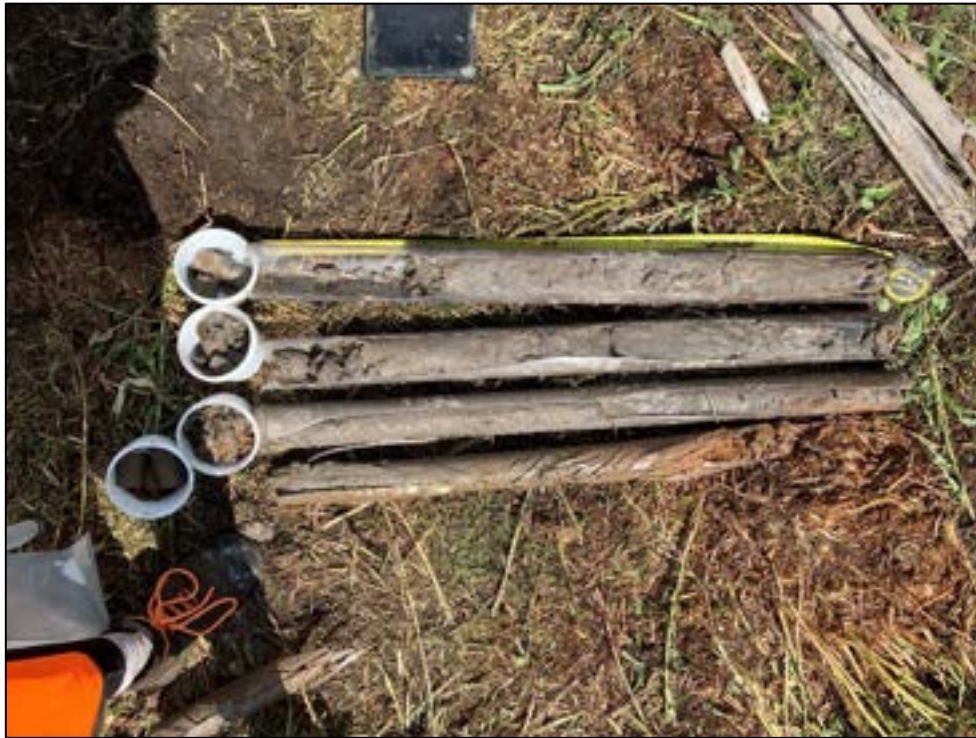
Photograph 40 – Photograph of the Hummocky Glacial Deposits between 1.2 – 5.45m depth bgl in WS04.
