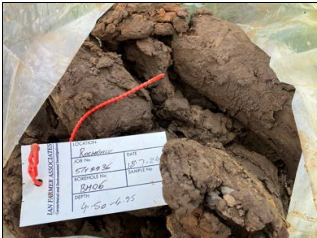
Photograph 18 – Photograph of the Hummocky Glacial Deposits between of 4.5 – 4.95m bgl in BH06.
