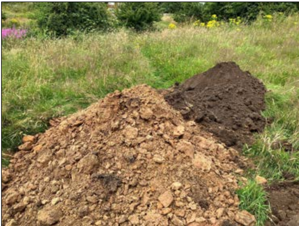
Photograph 69 – Photograph of TP25 arisings with Hummocky Glacial Deposits left, and Topsoil right.
