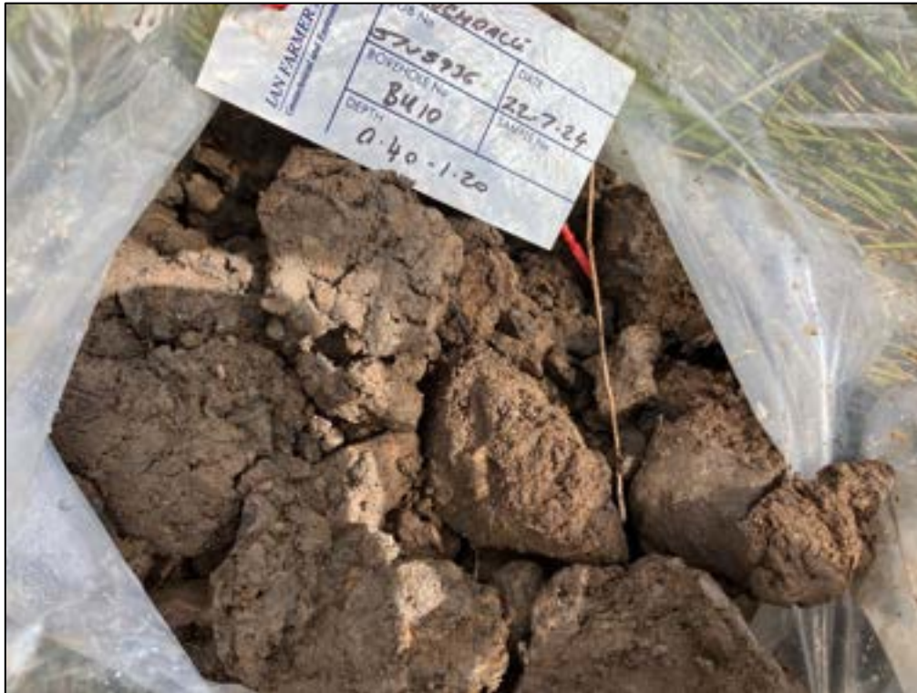
Photograph 27 – Photograph of the Hummocky Glacial Deposits between 0.4 – 1.2m depth bgl in BH10.
