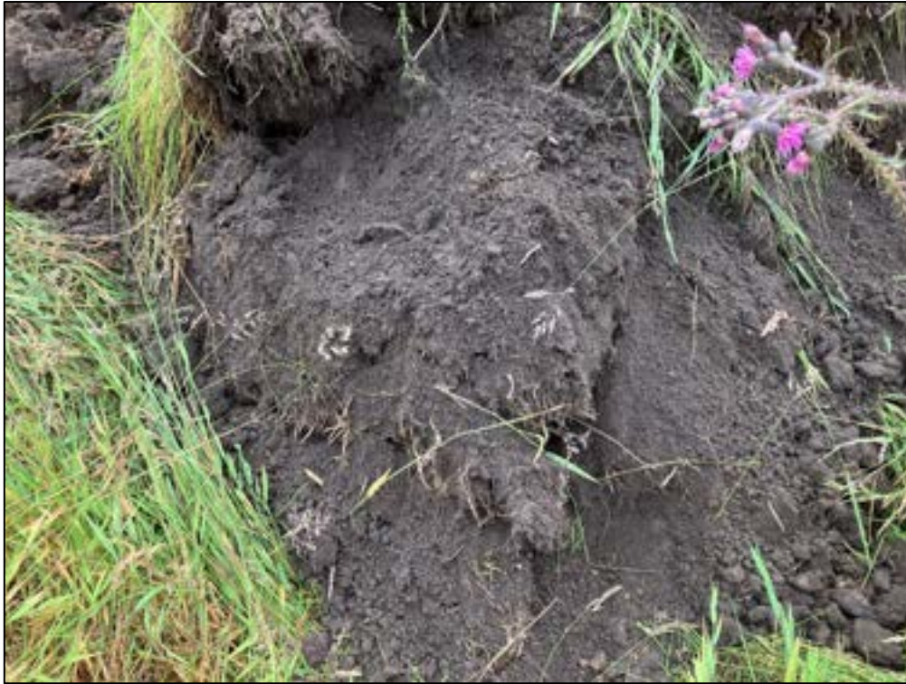
Photograph 11 – Photograph of the Topsoil encountered in TP04.
