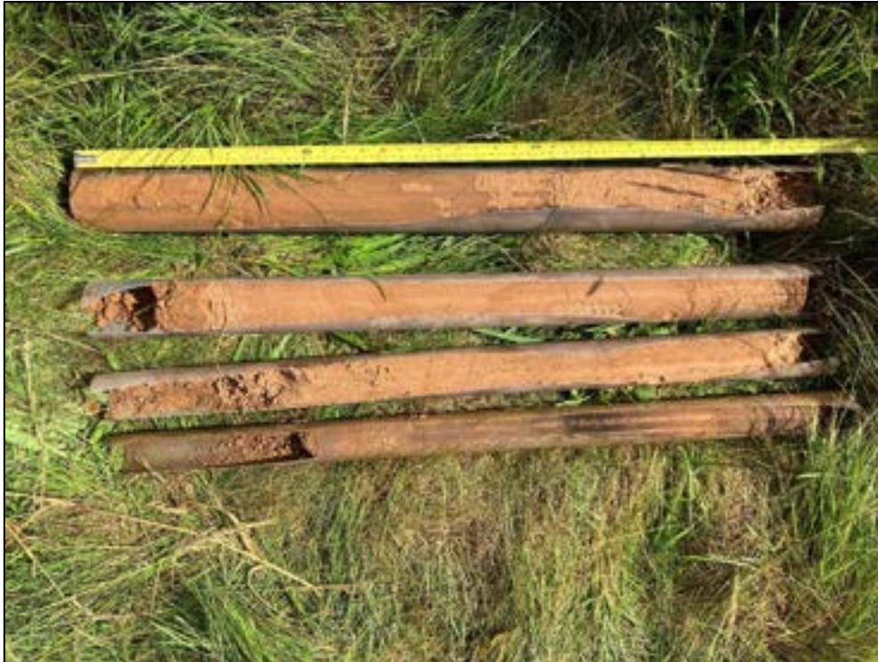
Photograph 34 – Photograph of the Hummocky Glacial Deposits between 1.2 – 5.0m in WS01.
