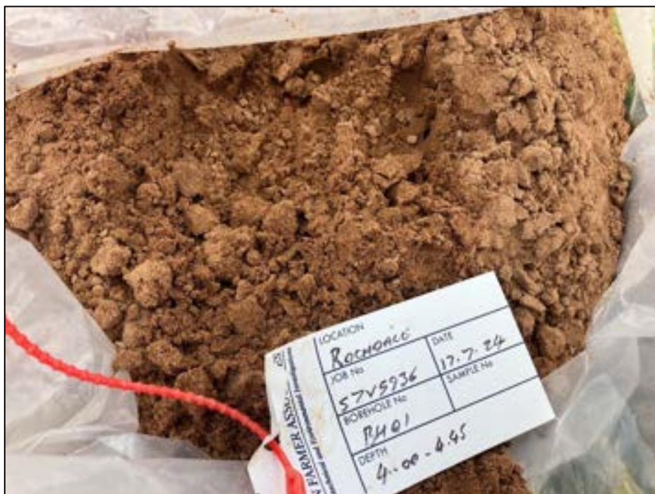
Photograph 2 – Photograph of the Hummocky Glacial Deposits between 4.0-4.45m bgl in BH01.
