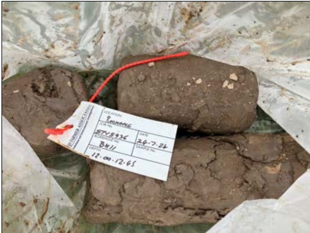
Photograph 31 – Photograph of the Hummocky Glacial Deposits between 12.0 – 12.45m depth bgl in BH11.
