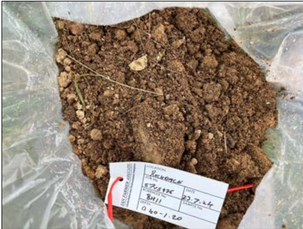
Photograph 29 – Photograph of the Hummocky Glacial Deposits between 0.4 – 1.2m depth bgl in BH11.
