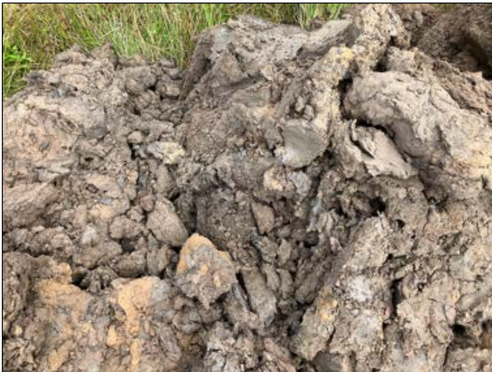
Photograph 26 – Photograph of the Hummocky Glacial Deposits encountered in TP09.
