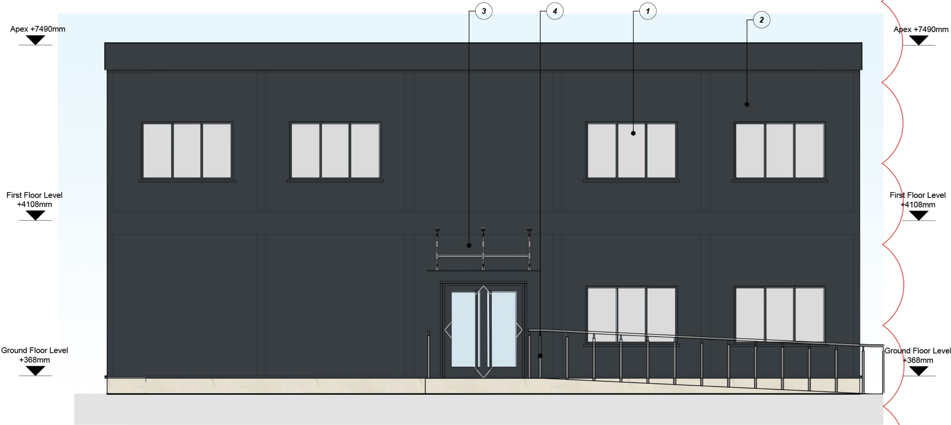
Amenity Building East Elevation Scale 1:50
