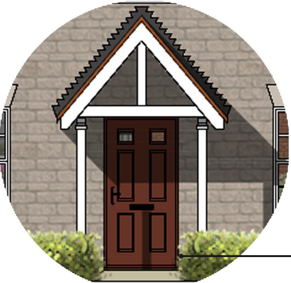
Feature entrance porch Individual formal 6 panel styled front door with ironmongery letterbox
