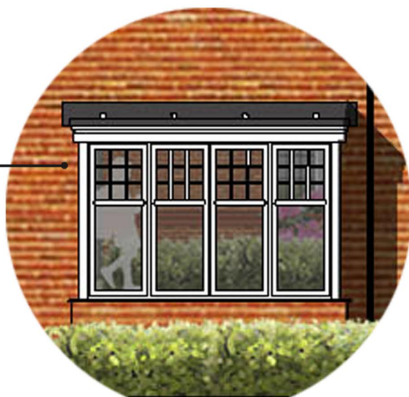
Square bay with lead rolled top roof
