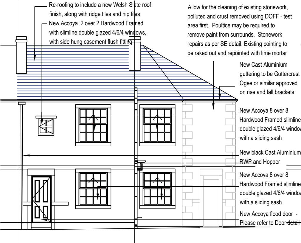
No2. Front Elevation as Proposed
