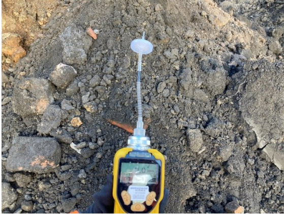
Plate 7 PID Screening of Odorous Soils
