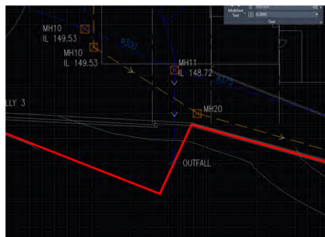
Surface water outfall on site
