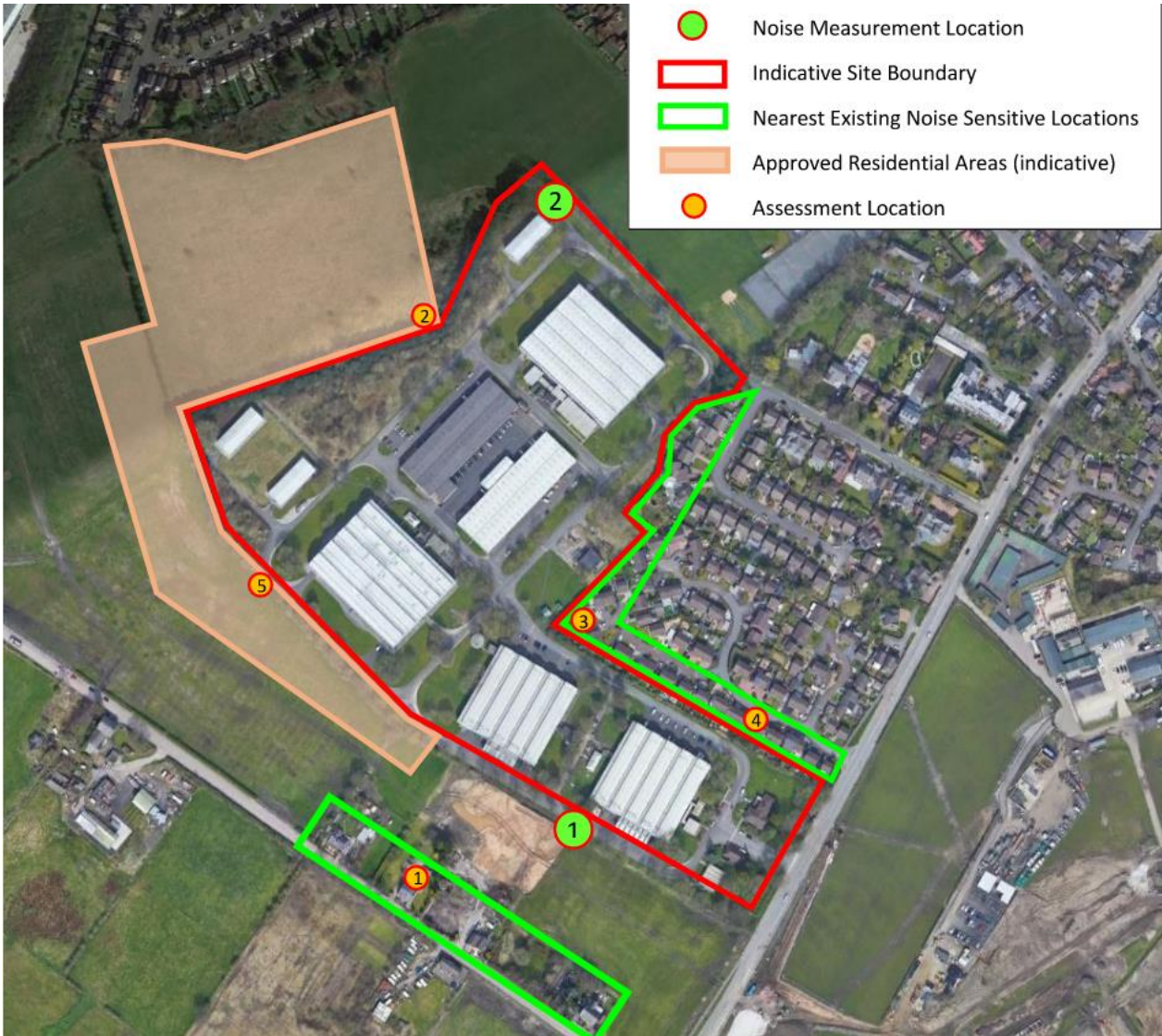
Figure 6-1: BWB Baseline Noise Survey Measurement Locations
