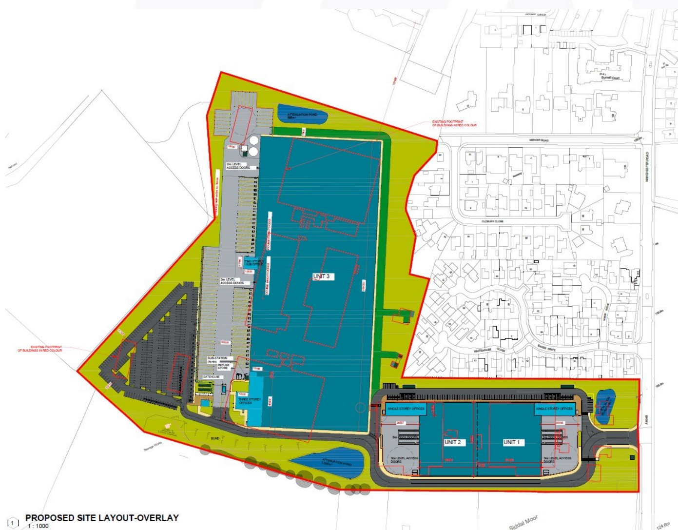
2.1.11 Each building's footprint is determined by numerous external factors, including: site constraints; the required access to and from the building; the activities required to operate the building; car parking requirements; service yard requirements (each building must have its own service yard); and maintenance access. 2.1.12 Units 1 and 2's design is cognisant of the existing building footprint layout (Fig 2). They use the same eastern building line as the existing and maintain a minimum of 30m distance to nearest dwelling. The boundaries are supplemented with additional planting and a new closed boarded fence. 2.1.13 For reference the proposed building footprint is 42,635m 2 and the un-developed area is 68,885m 2 . This clearly demonstrates that built area is appropriate in relation to undeveloped areas and that the scheme does not represent overdevelopment.
