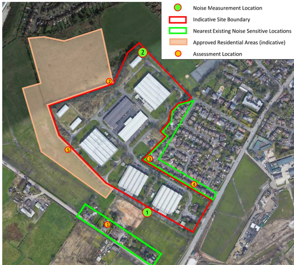
Figure 56-1: BWB Baseline Noise Survey Measurement Locations
