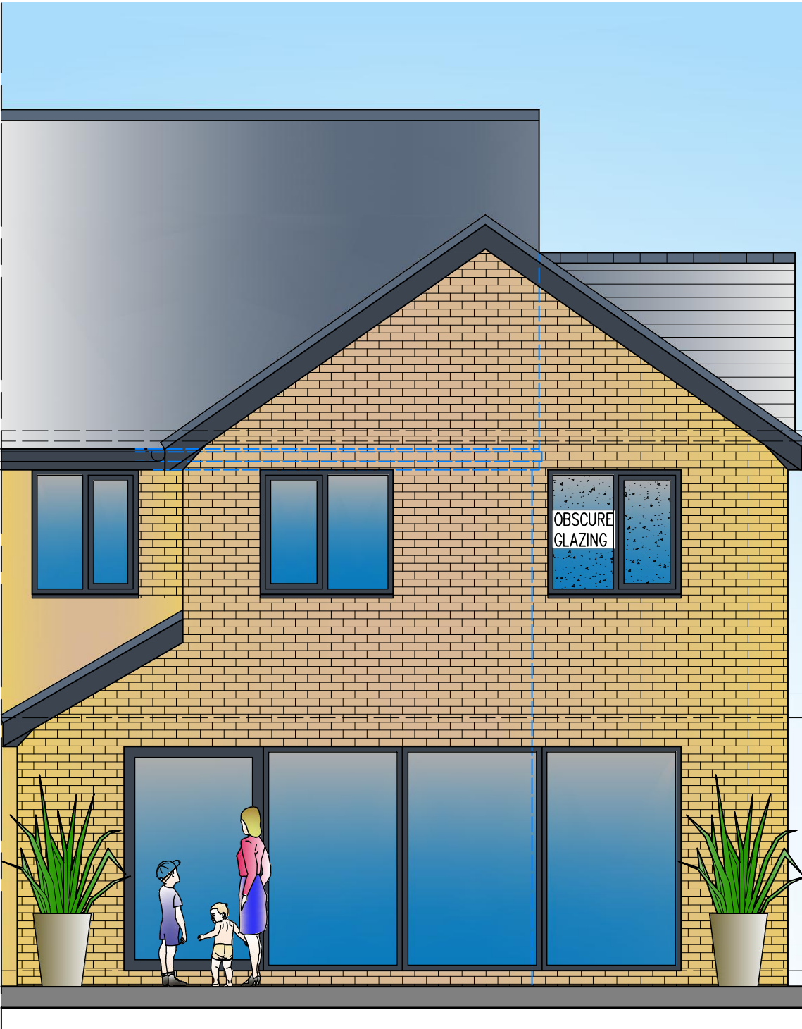
PROPOSED REAR ELEVATION scale 1:50
