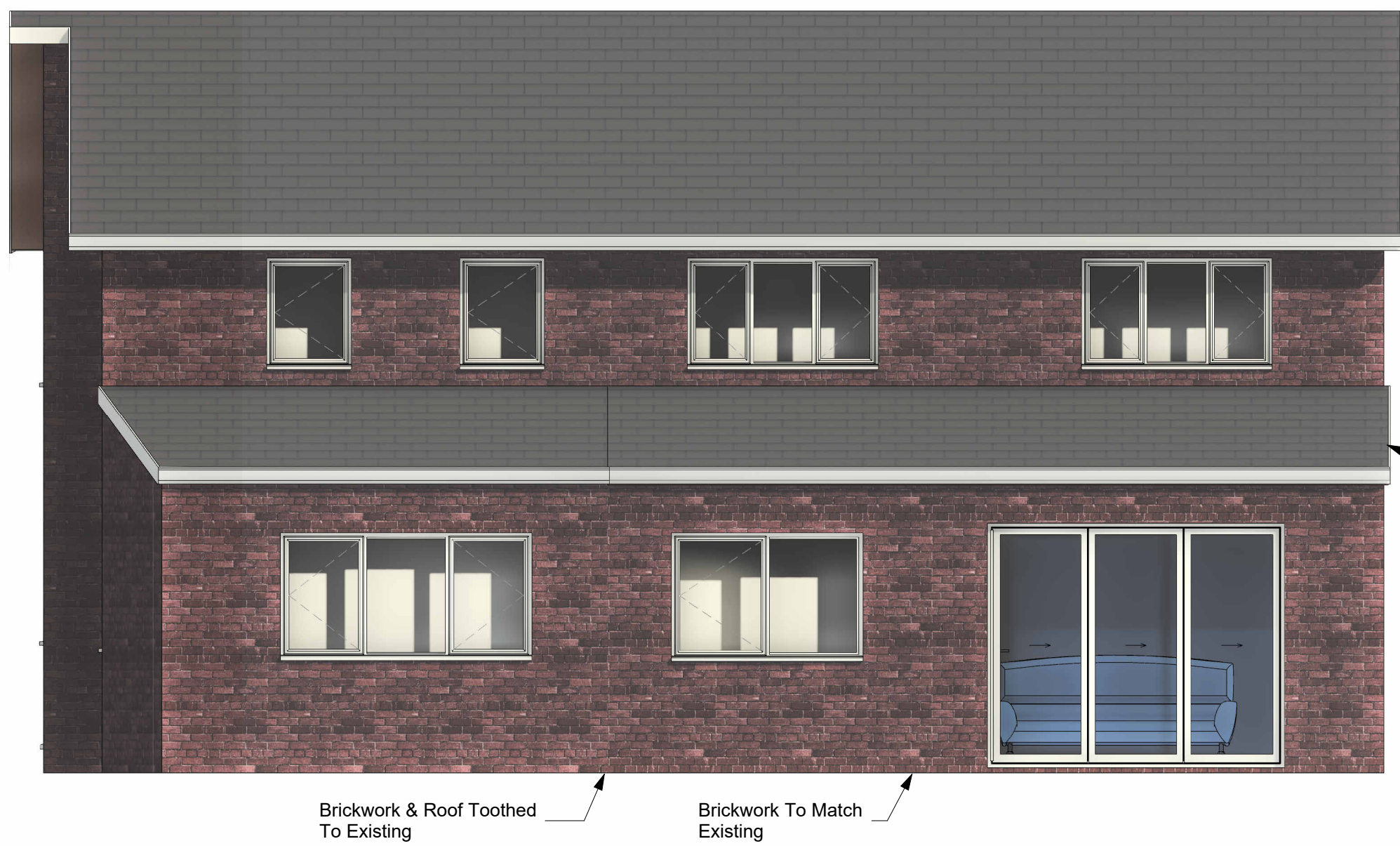
4 Proposed Rear Elevation 1 : 50
