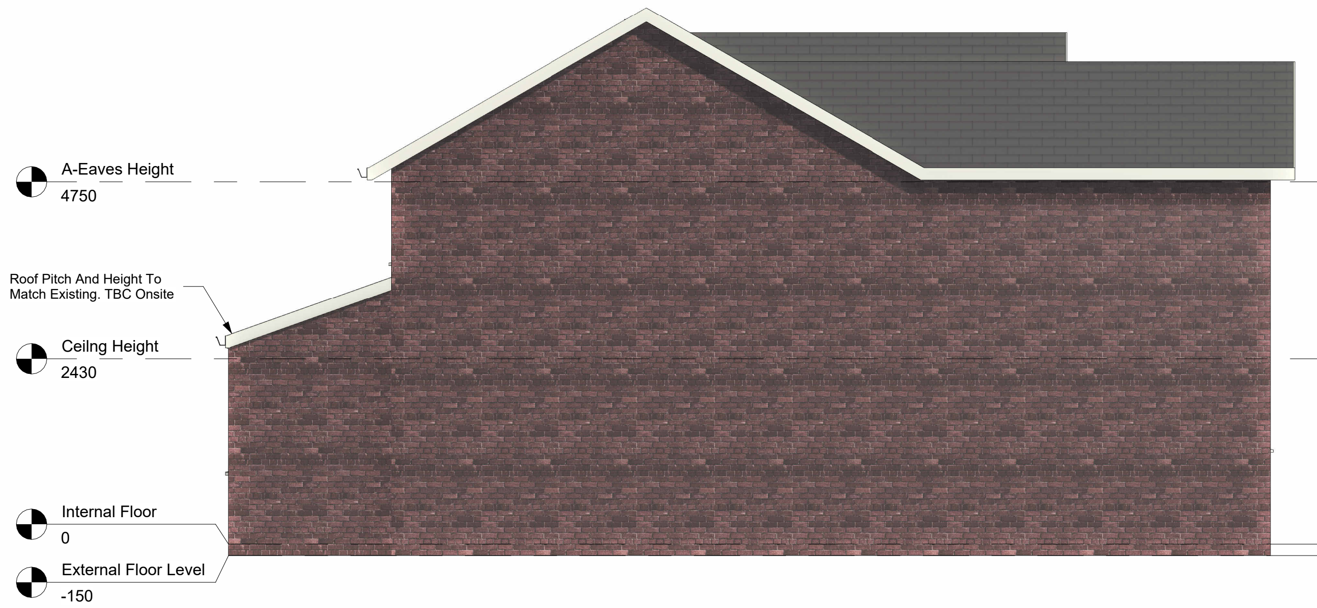
3 Proposed LHS Gable Elevation 1 : 50
