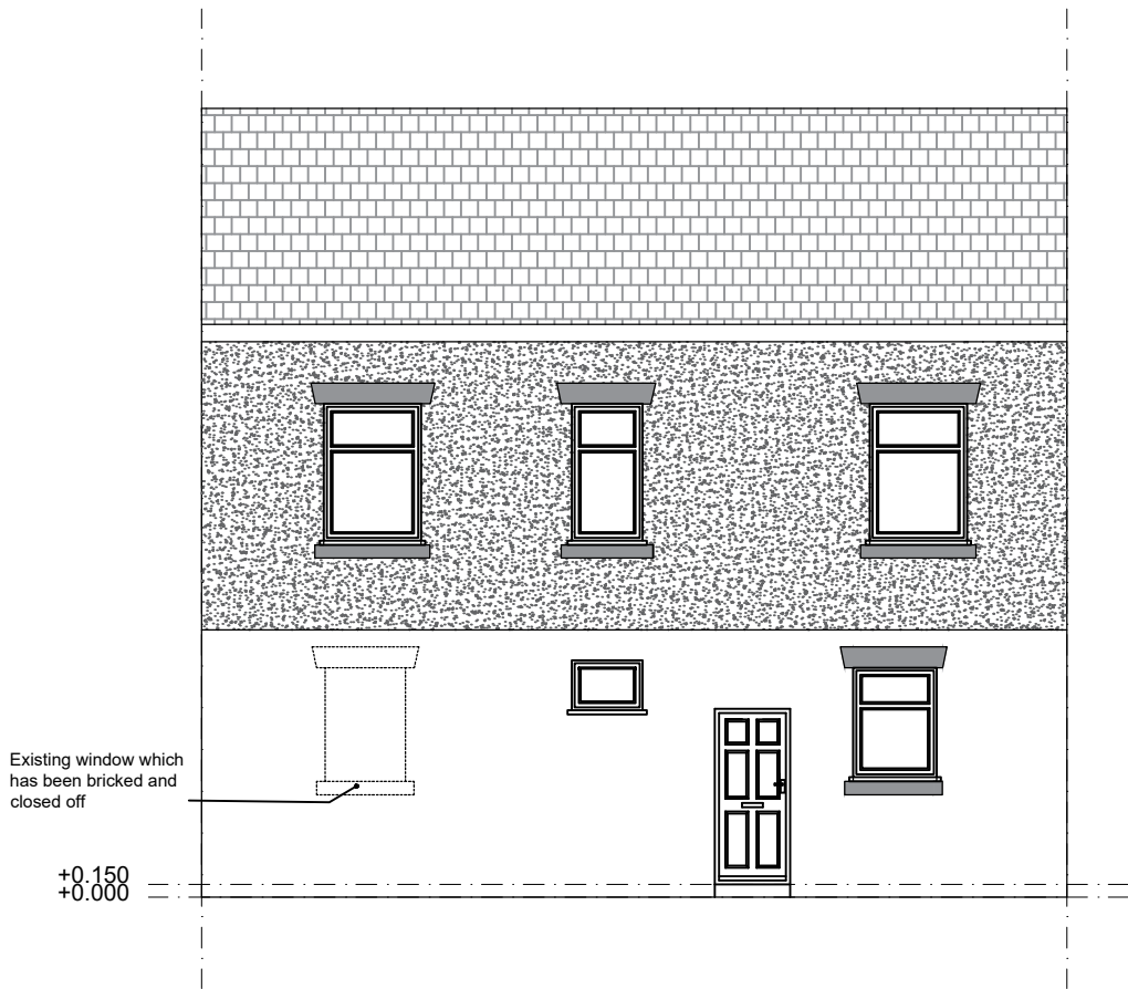
Existing Rear Elevation
