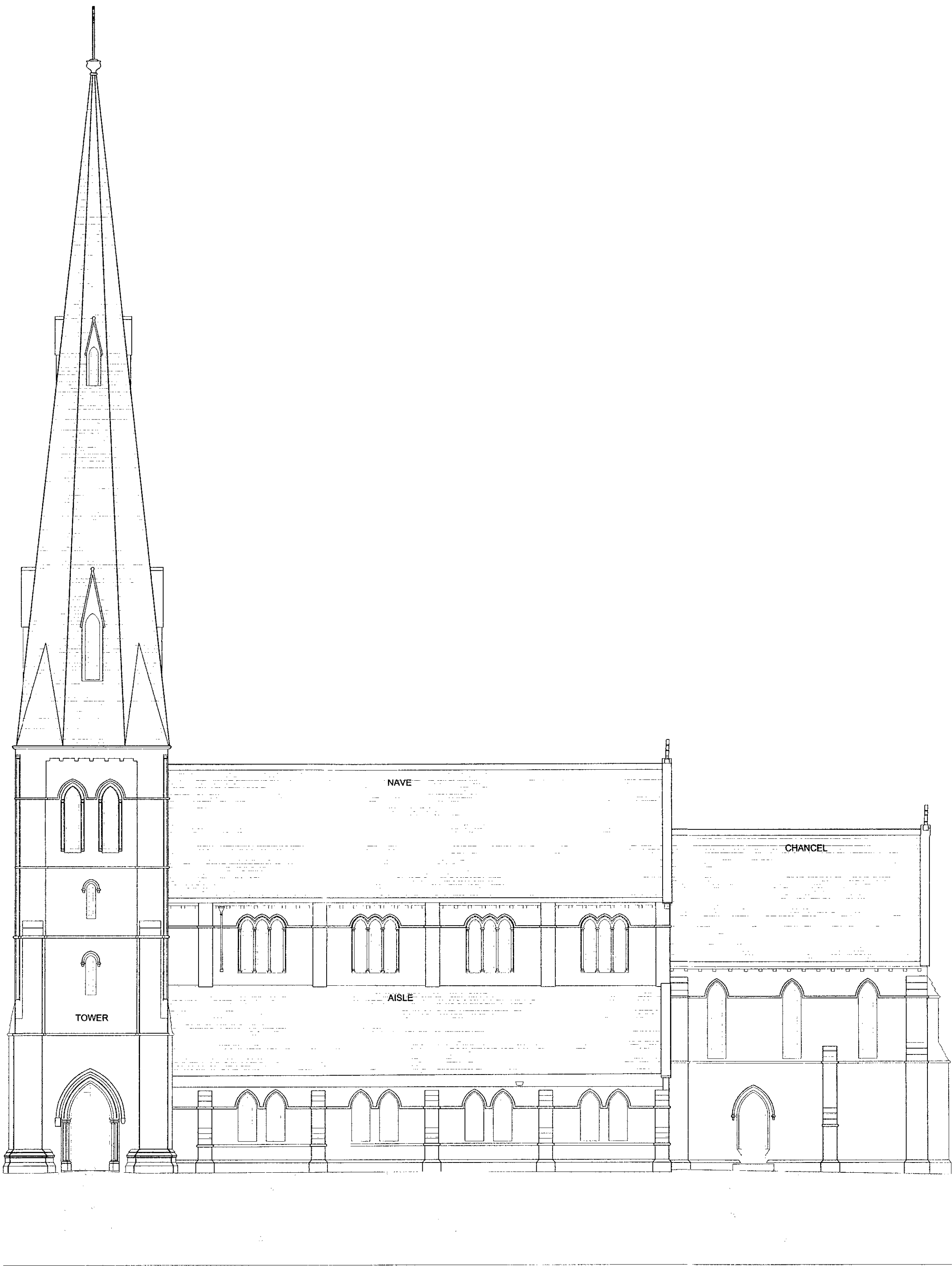
ELEVATION 2 SOUTH ELEVATION
