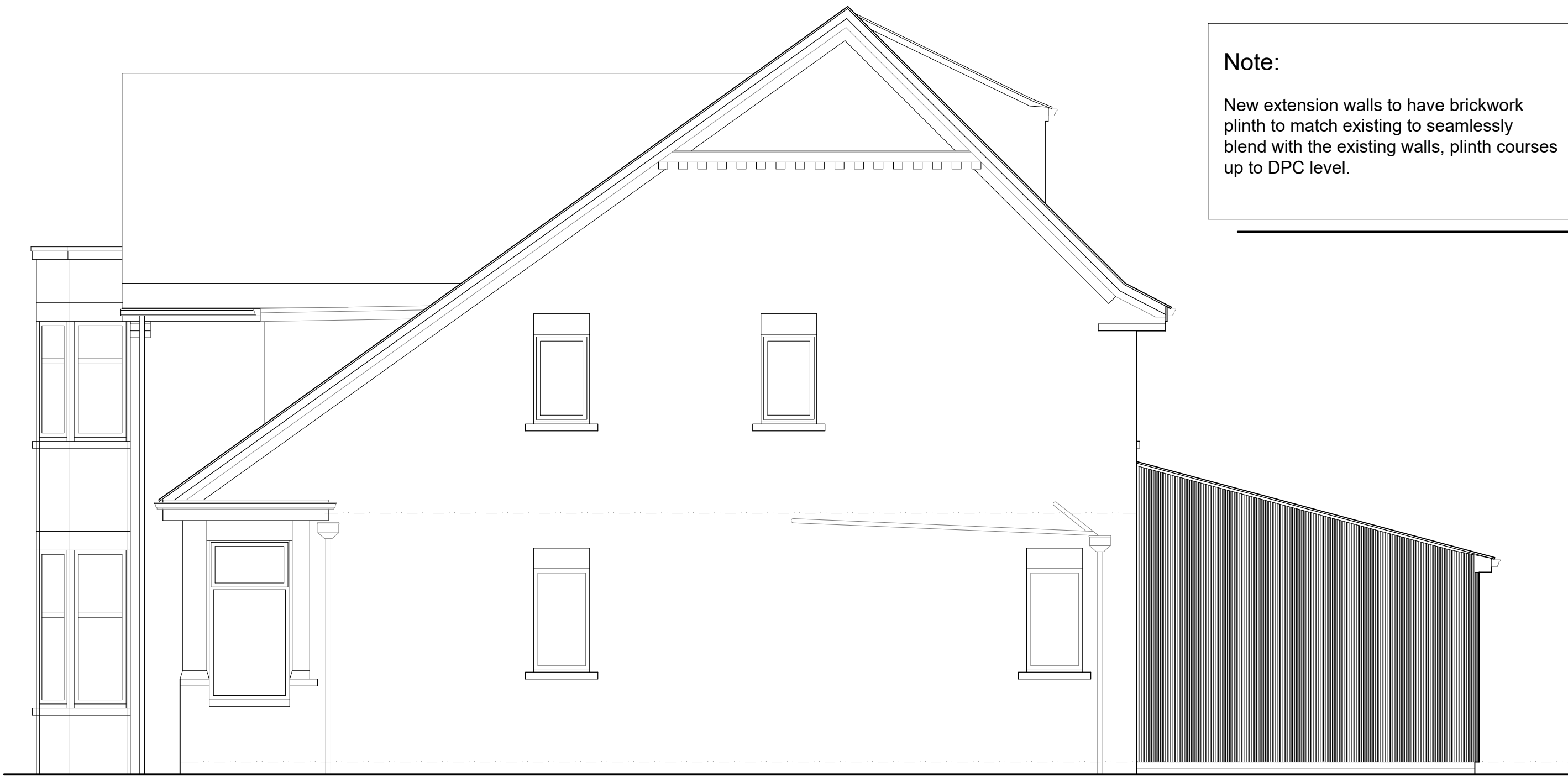
SIDE ELEVATION (NORTH WEST)
