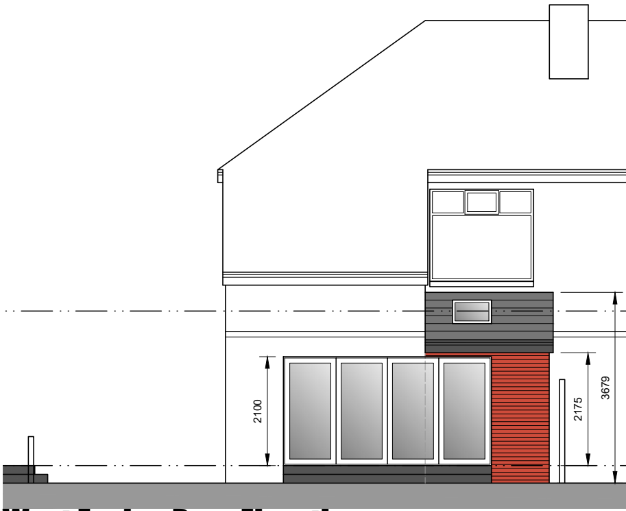
West Facing Rear Elevation
