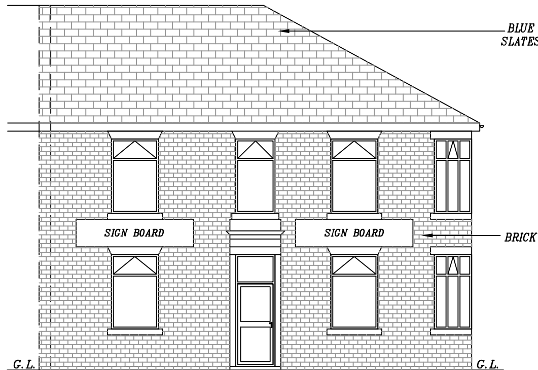
EXISTING FRONT ELEVATION
