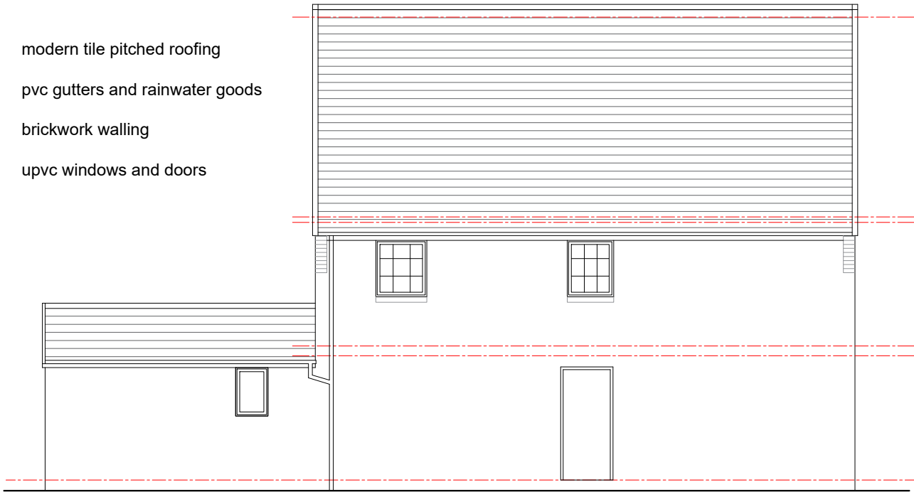
north west elevation
