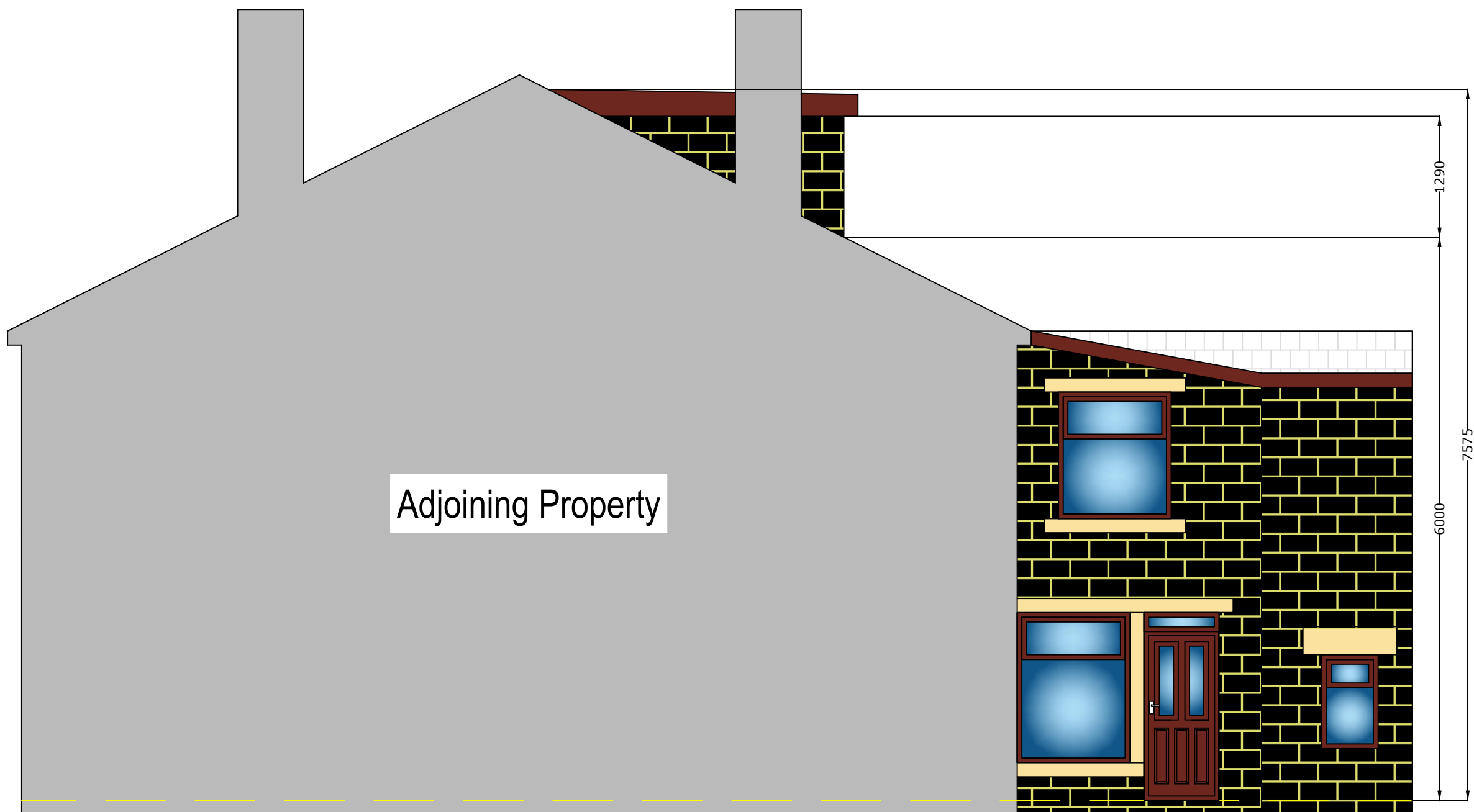
Proposed (RHS) Gable Elevation
