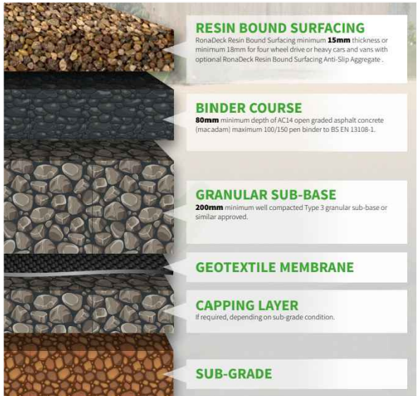
Grey Bound Resin Build Up Detail
