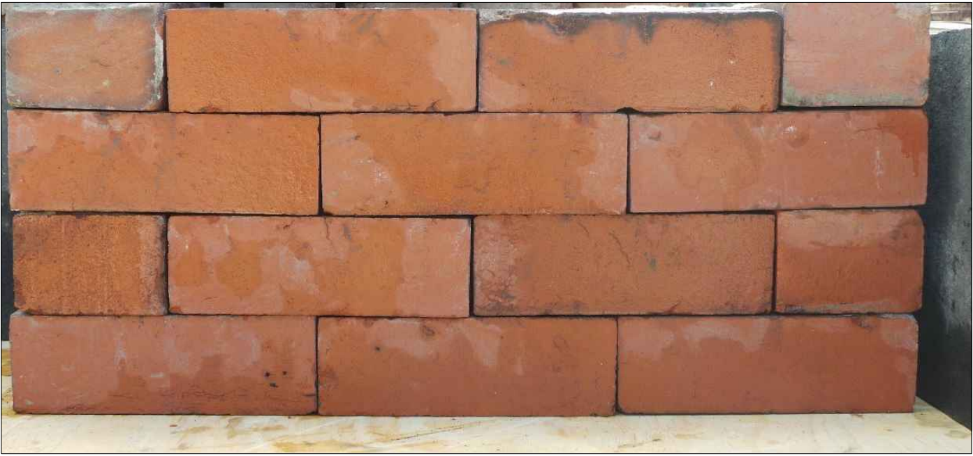
Proposed reclaimed Accrington brick to be used for blocking up window openings
