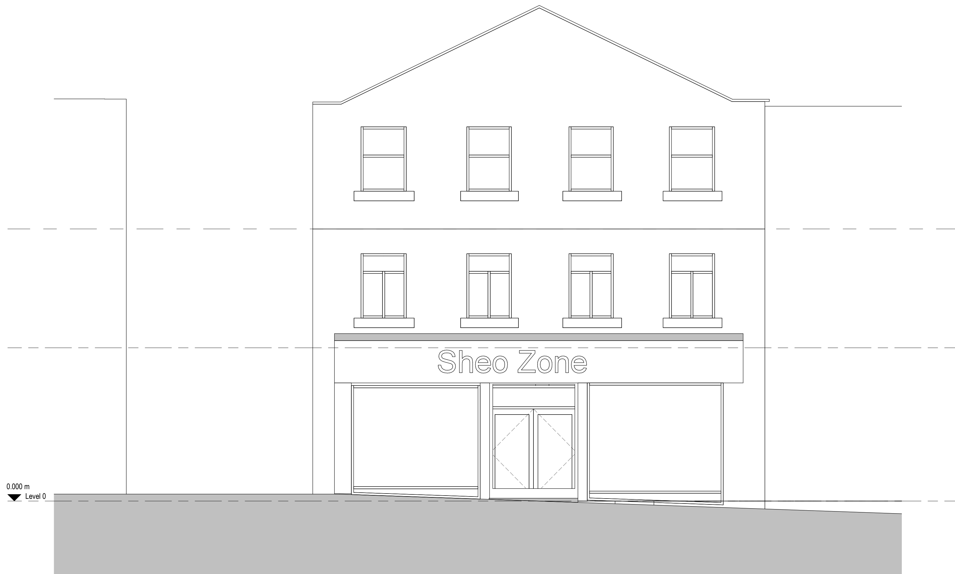
2 Existing Front Elevation 1 : 50
