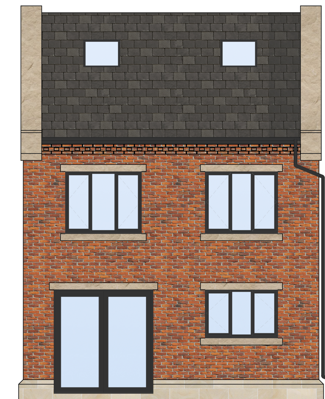
PLOT 3 REAR ELEVATION AS PROPOSED (1:50)
