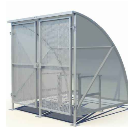
GALVANISED STEEL FRAMED CYCLE STORAGE SHELTER, FOR 10 CYCLES, 2150mm WIDE x 2900mm LONG x 2200mm HIGH, GATED FRAMES TO RECEIVE PERFORATED INFILL PANELS. PROVIDE 5mm SHEET PILING STANDS, FIXED TO TO HARD STANDING.
