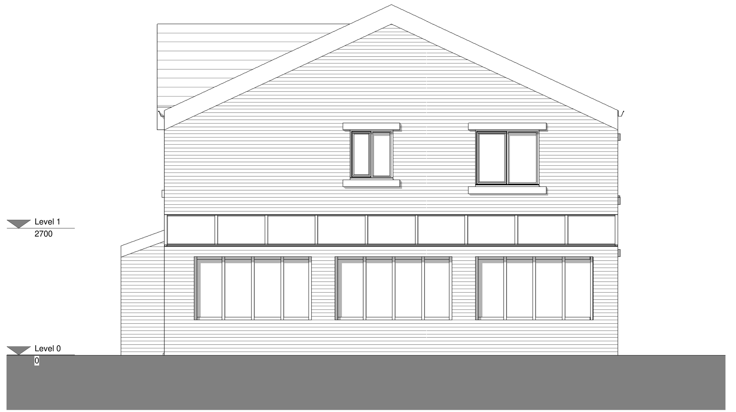
4 Existing East Elevation 1 : 50
