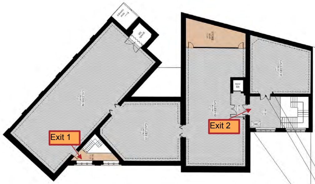
Figure 7 Storey Escape at First Floor
