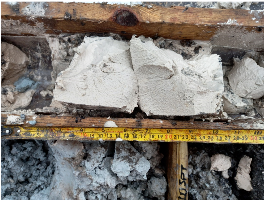
Photograph 15 — BH02; Close up of sample within 1.25 – 2.00m run
