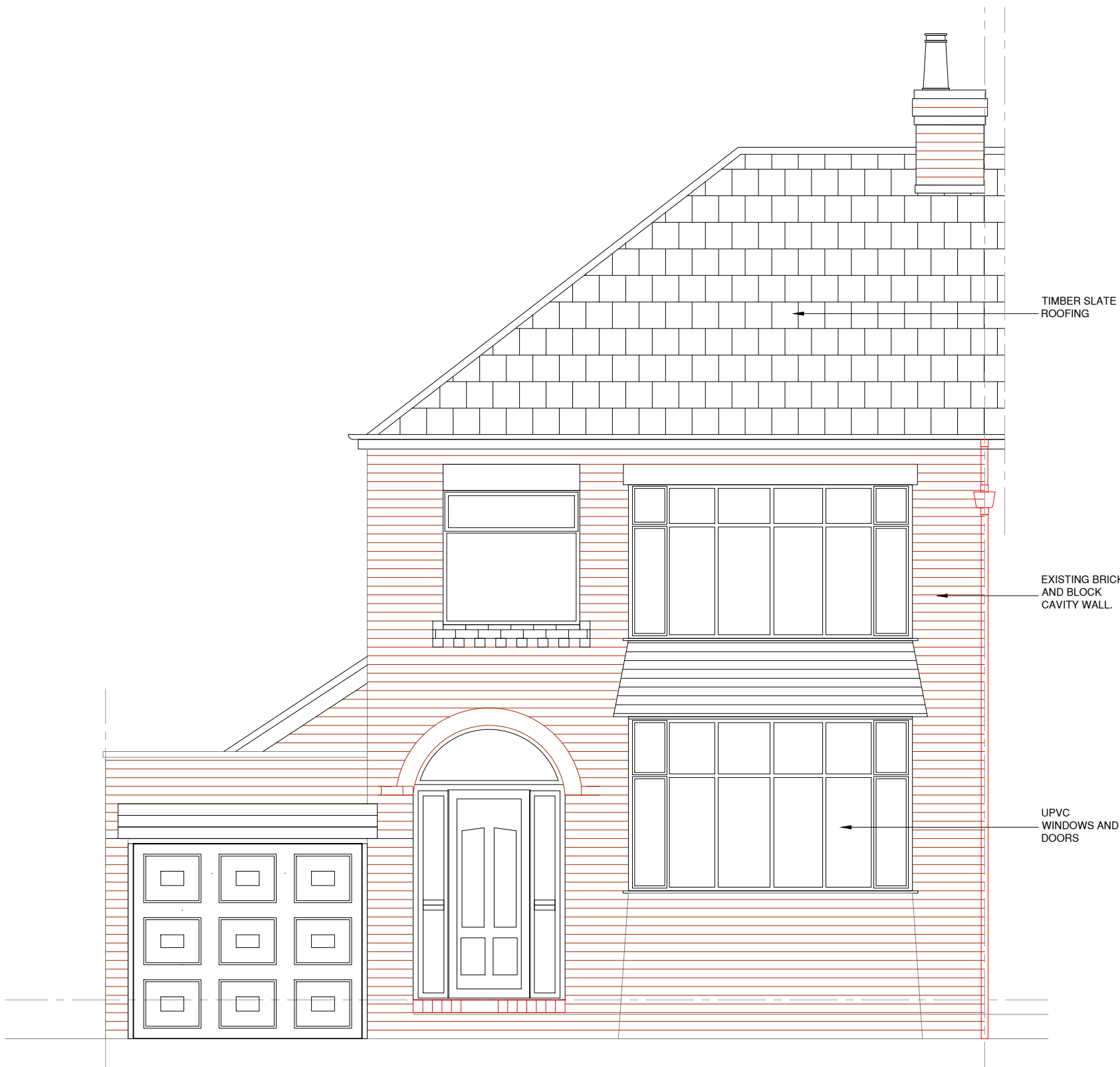
EXISTING FRONT ELEVATION
