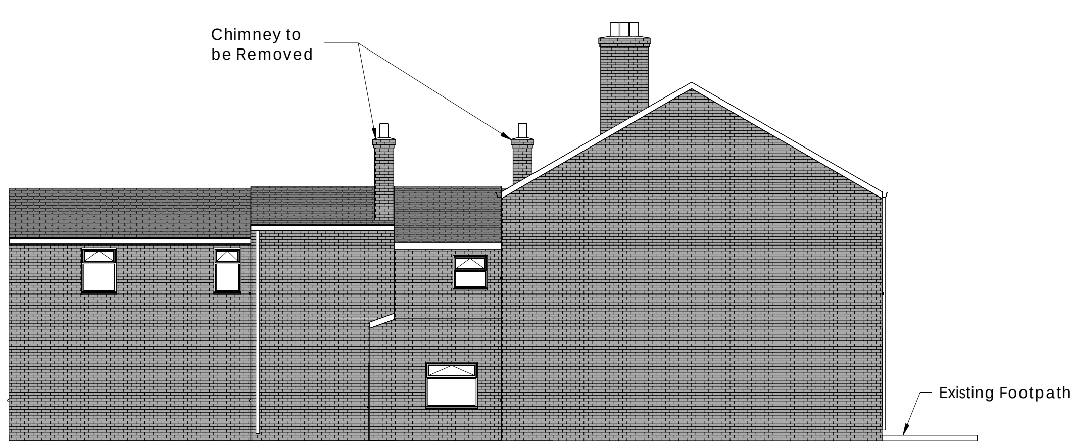
4 Existing Wast Elevation
