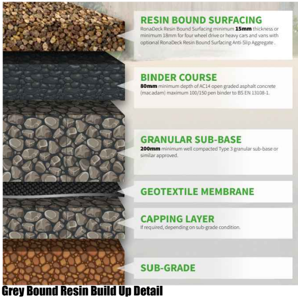
Grey Bound Resin Build Up Detail
