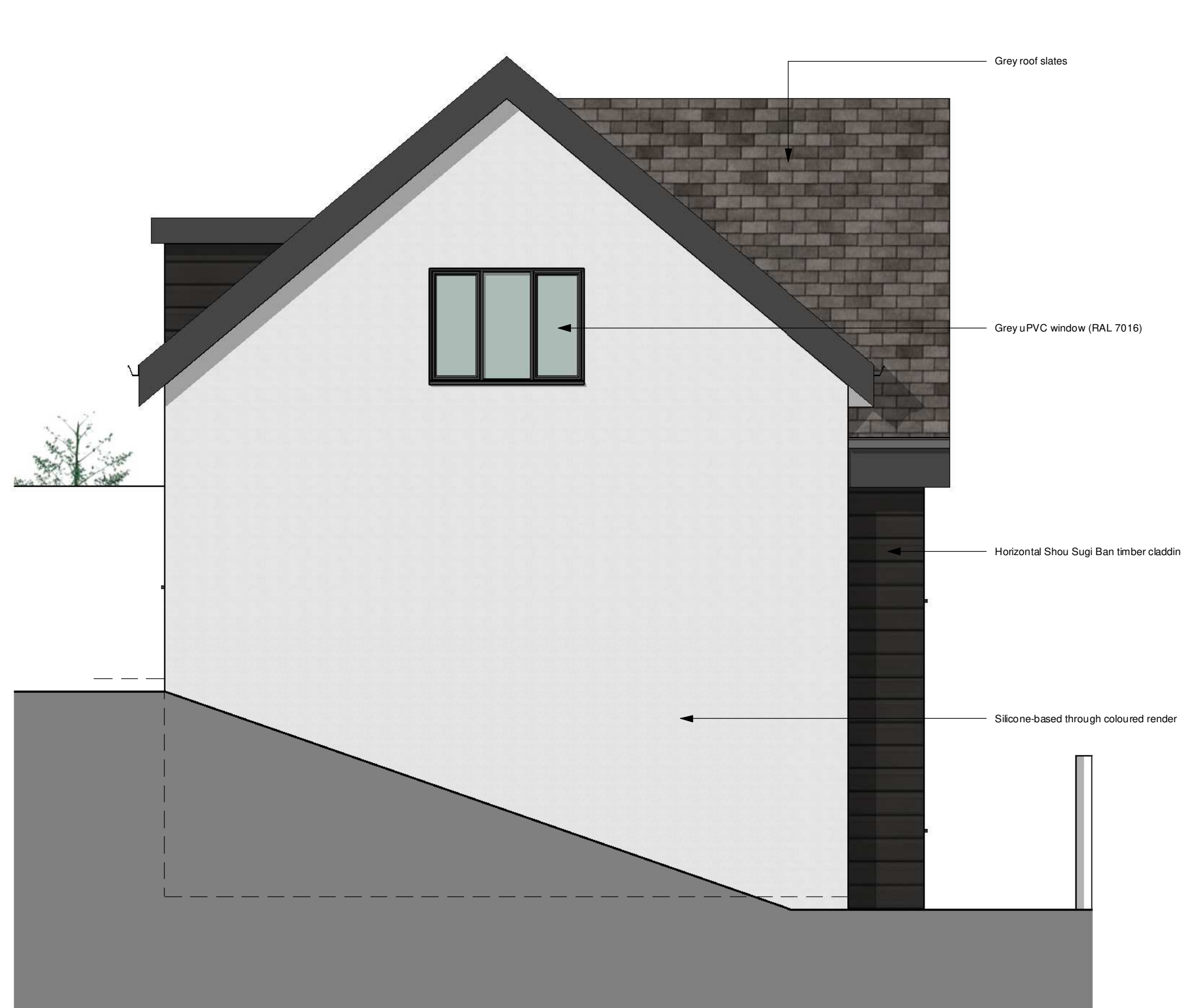
Proposed East Elevation 1 : 50
