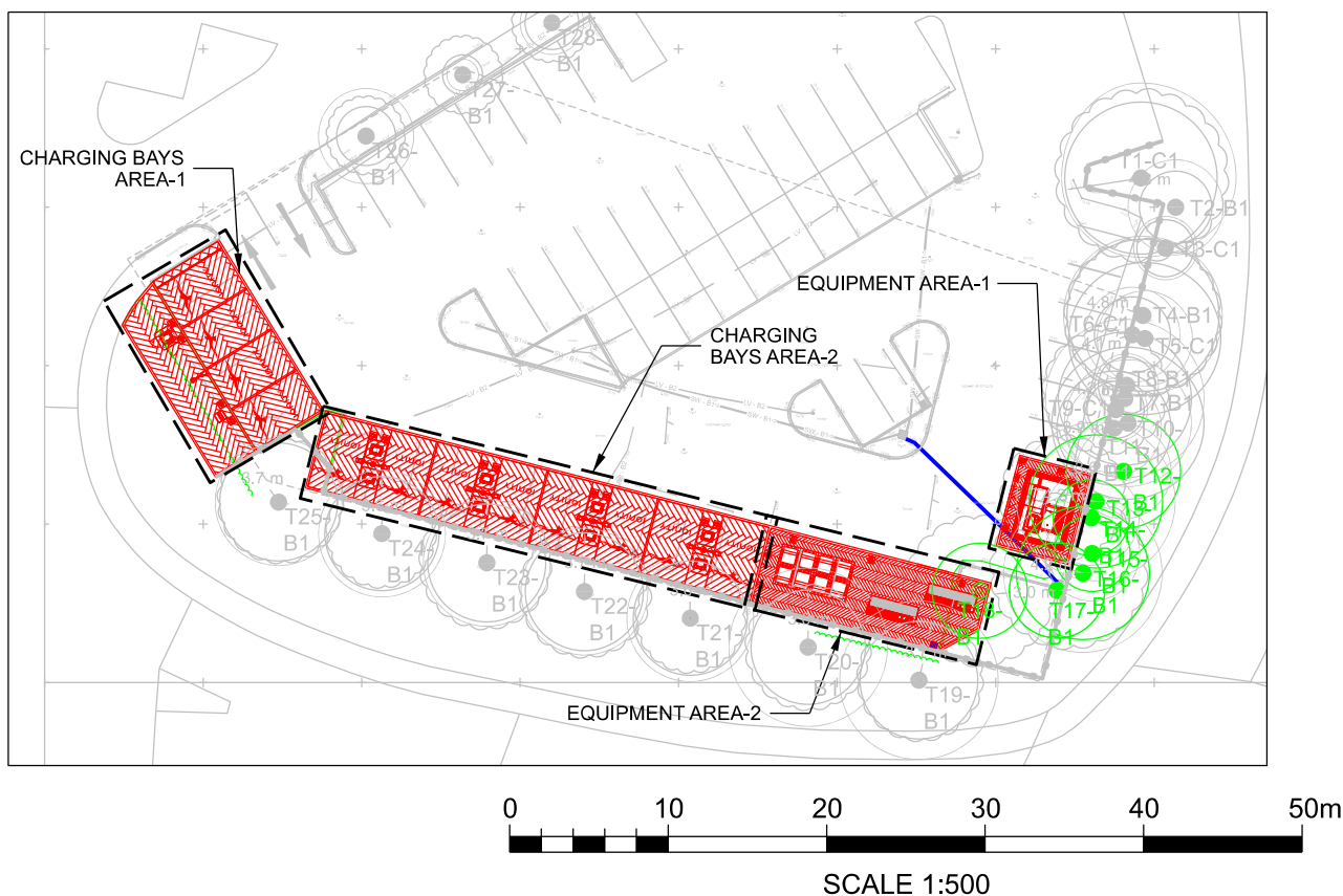
EV BAYS AND EQUIPMENT AREA PLAN SCALE 1:500
