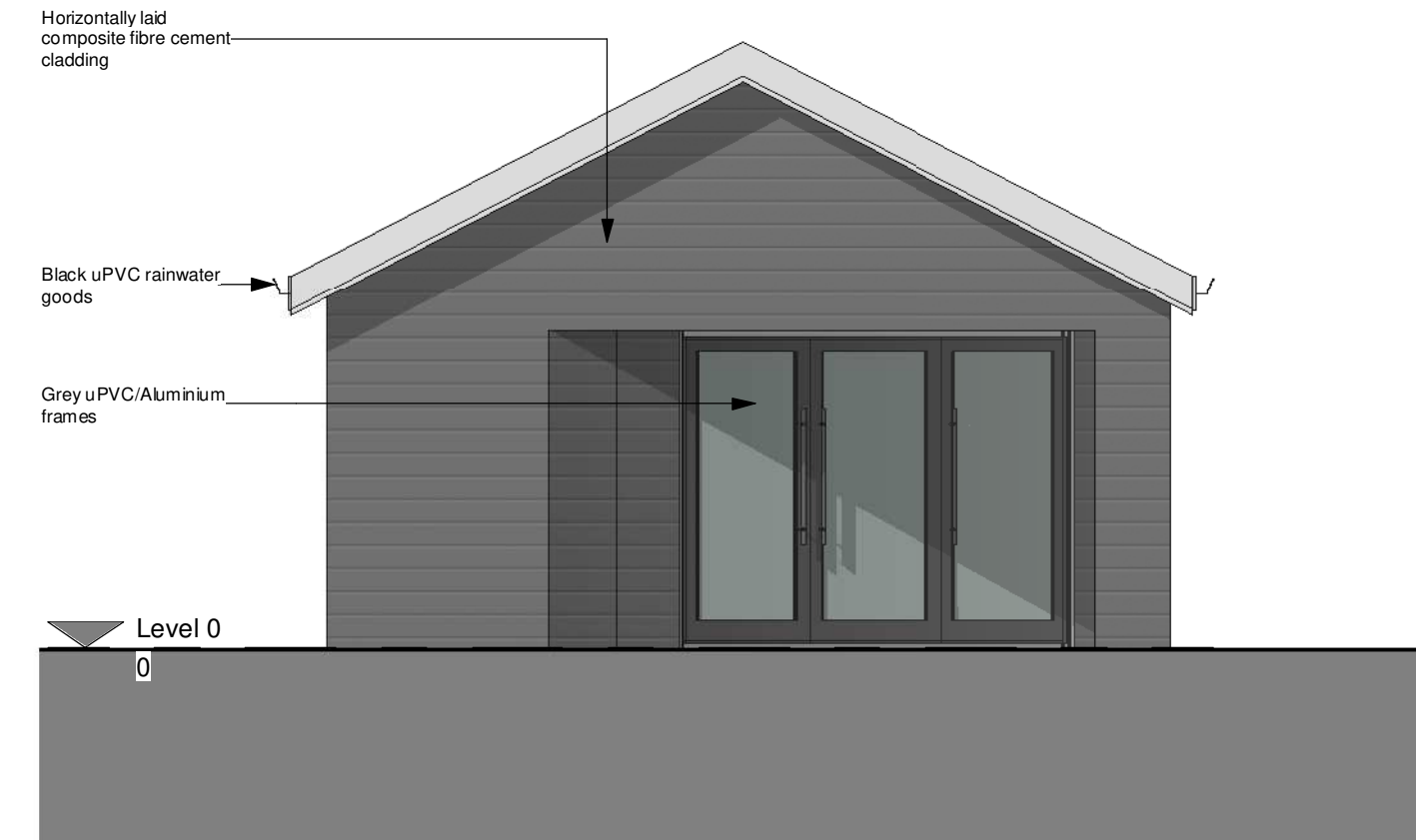
2 | PRO Outbuilding East Elevation 1 : 50
