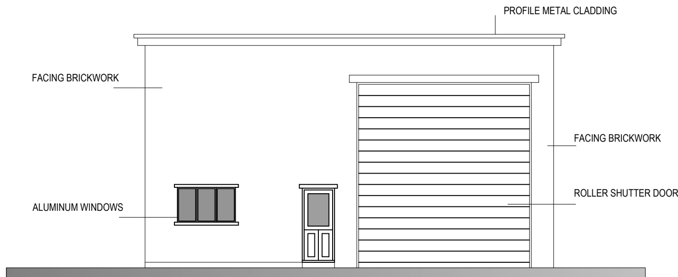
PROPOSED FRONT ELEVATION
