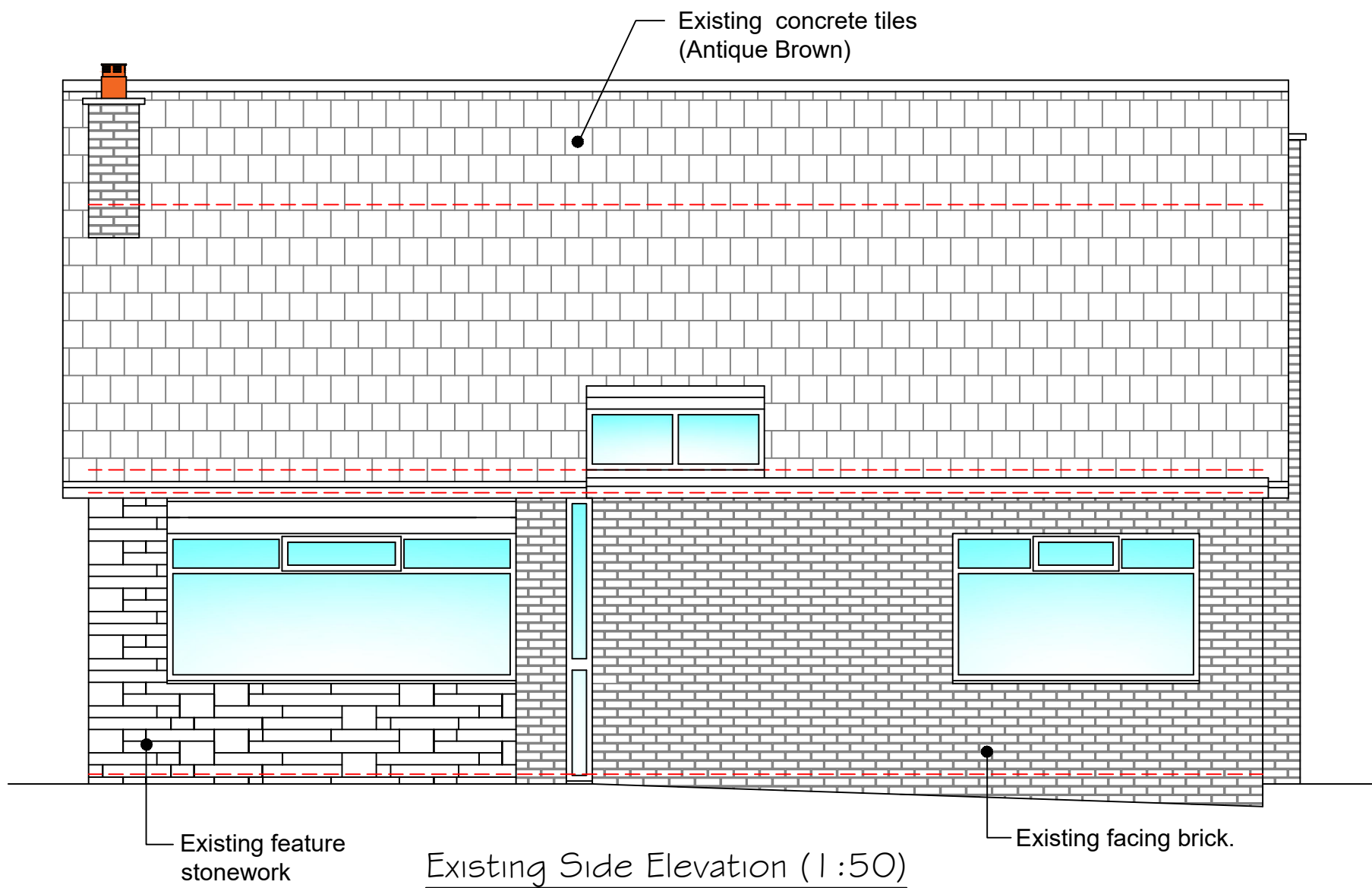
Existing Side Elevation (1:50)
