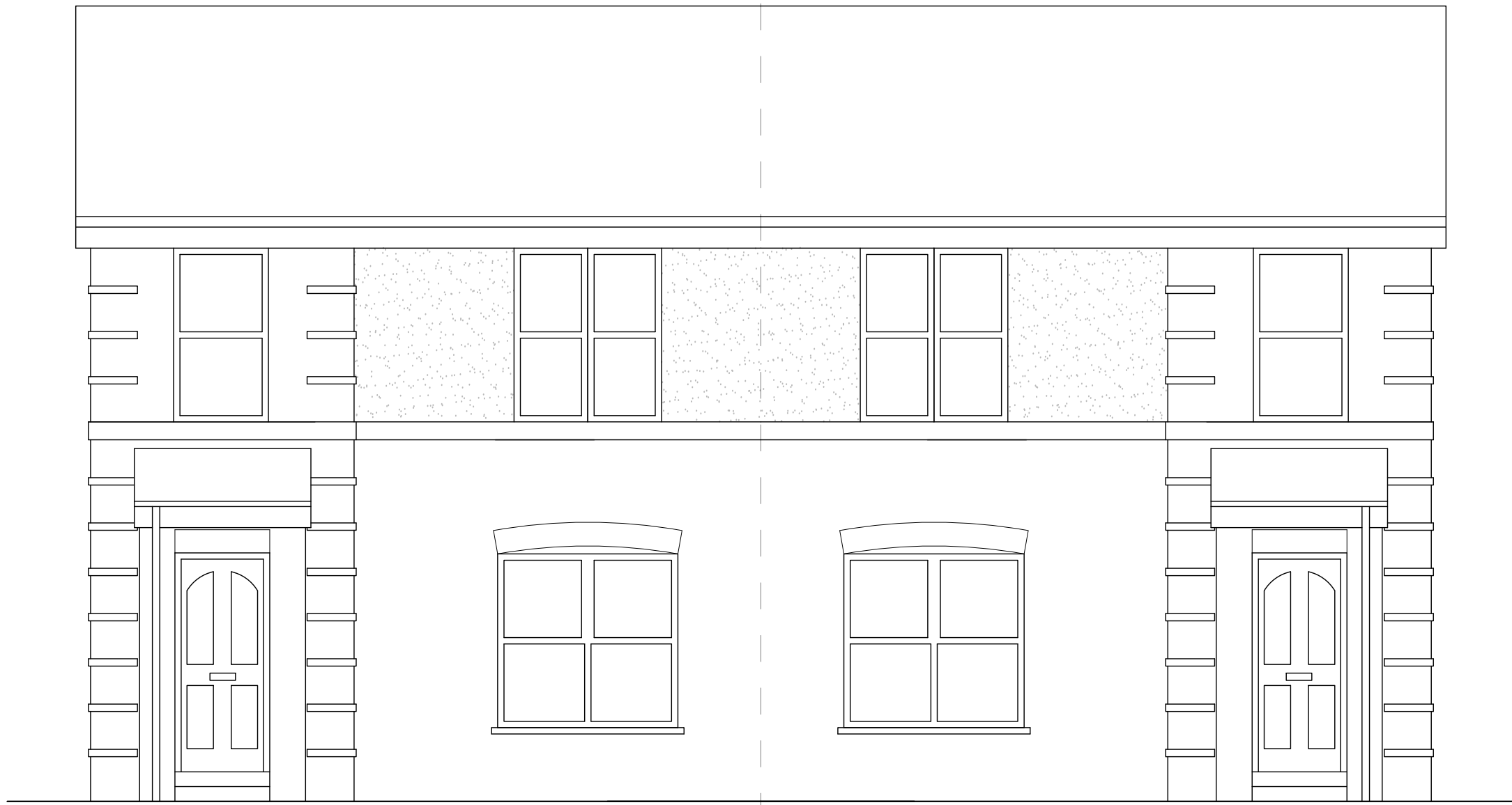
House type A - semi-detached houses with slightly projecting facade around entrance. Brick construction with render to parts of first floor
