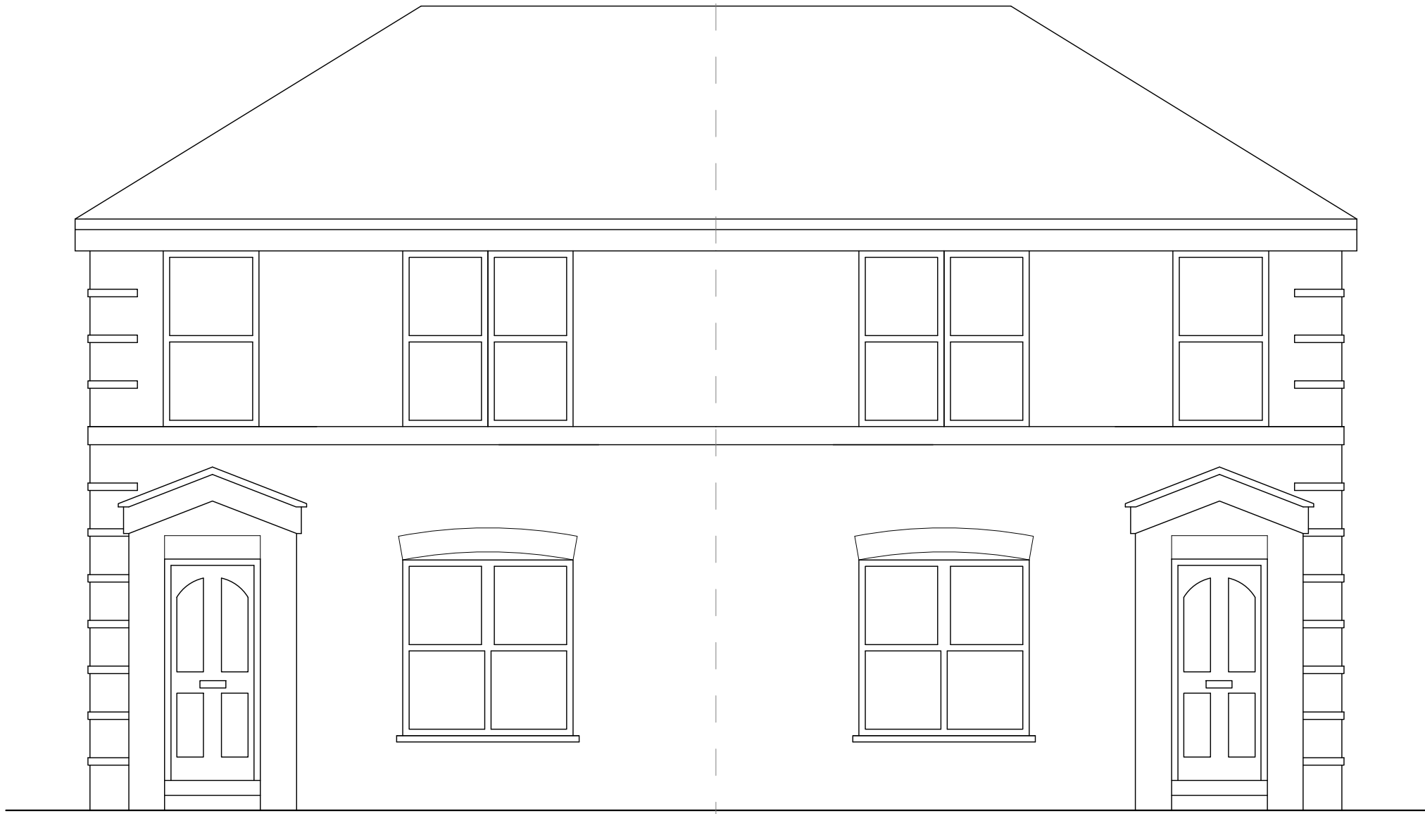
House type B - semi-detached houses with flat facade. All brick construction
