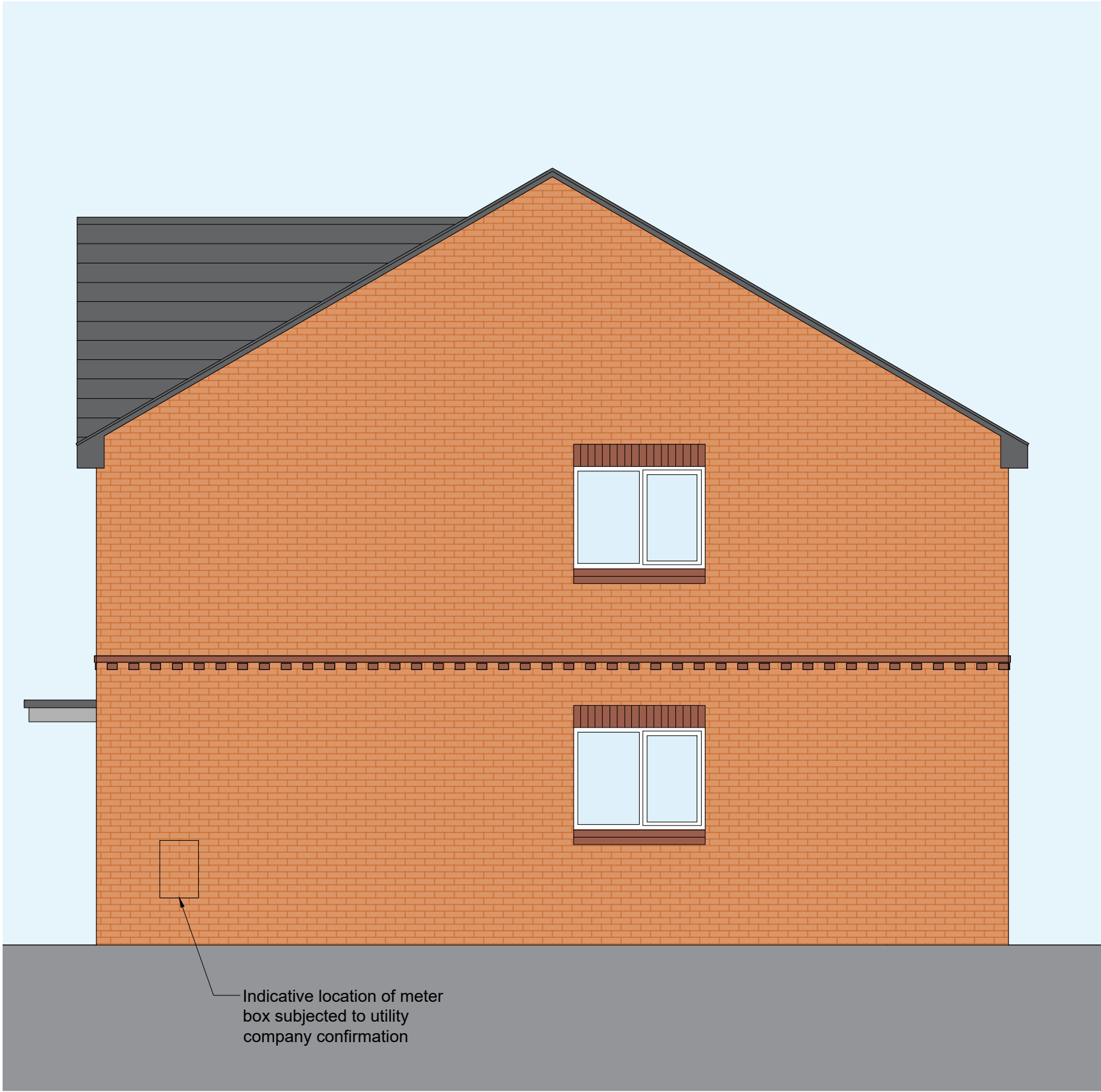
Proposed Plot 2 Gable Elevation Scale 1:50
