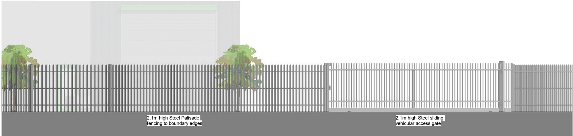
Street Elevation - Boundary Treatment - Scale 1:100@A3
