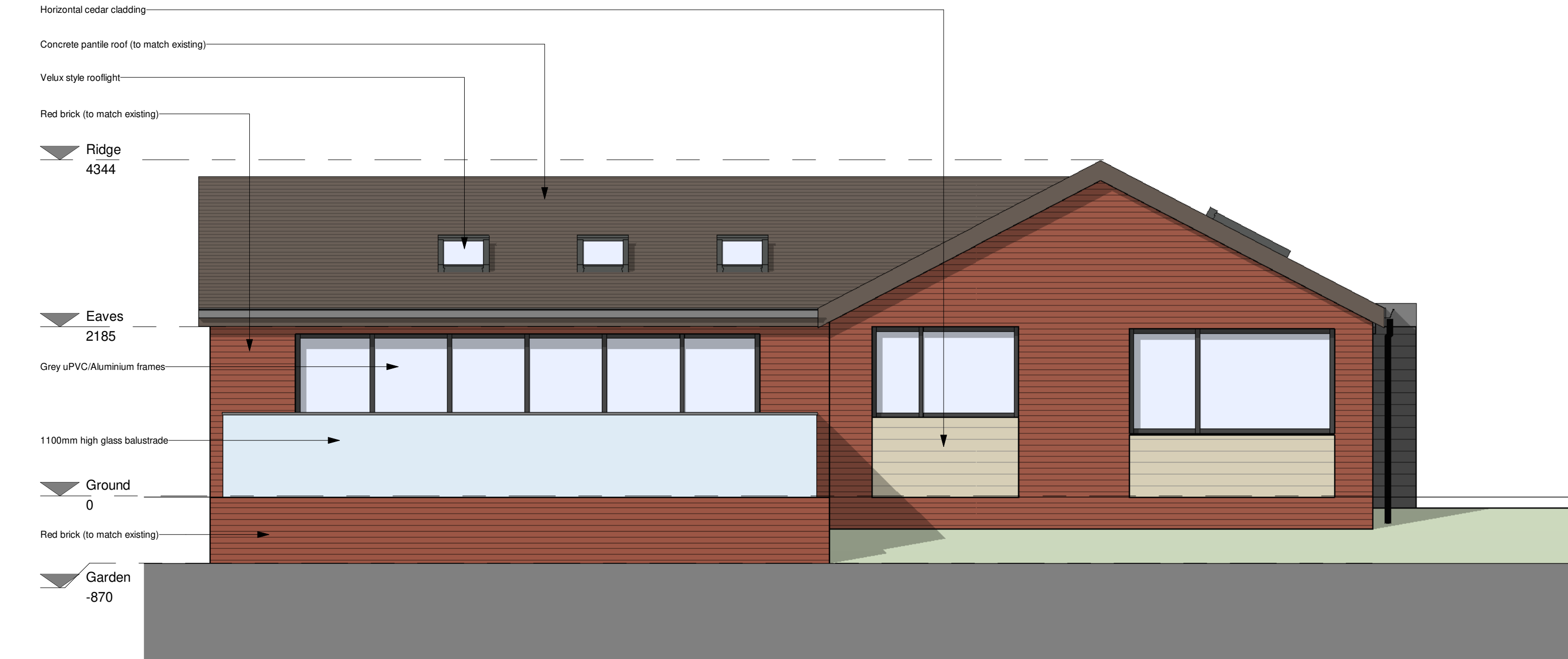
Proposed South Elevation 1 : 50
