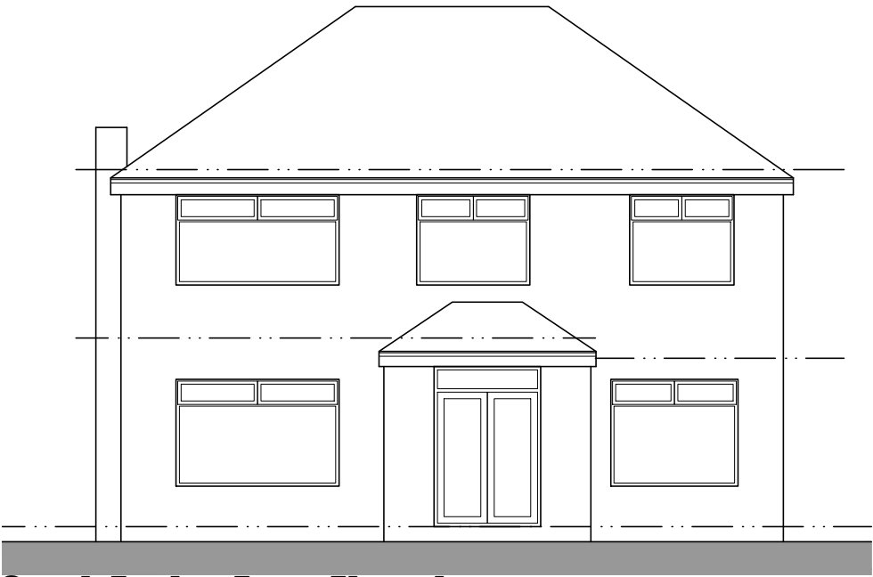
South Facing Front Elevation
