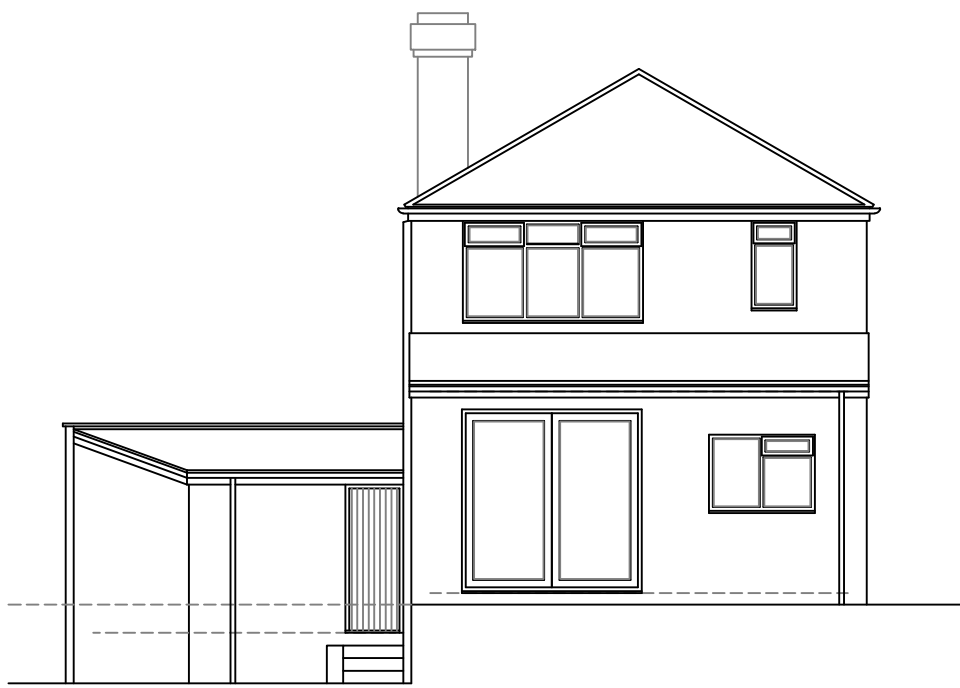
Existing Rear Elevation
