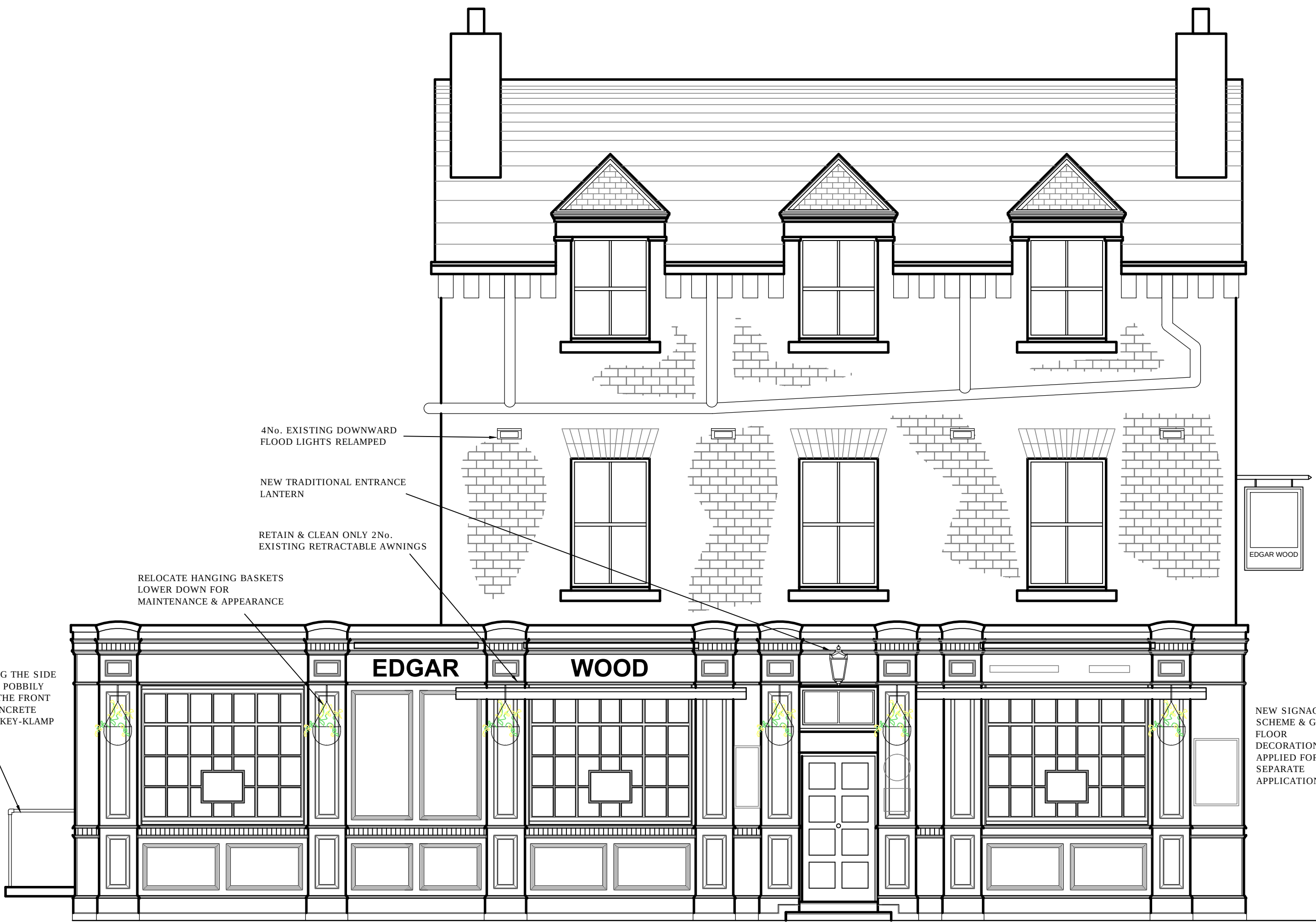
PROPOSED FRONT (SOUTH FACING) ELEVATION SCALE 1:50 @ A1
