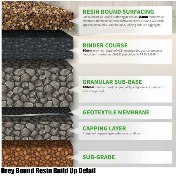
Grey Bound Resin Build Up Detail
