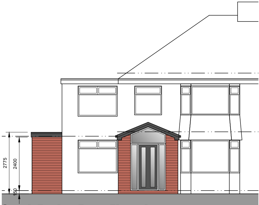
South Facing Front Elevation
