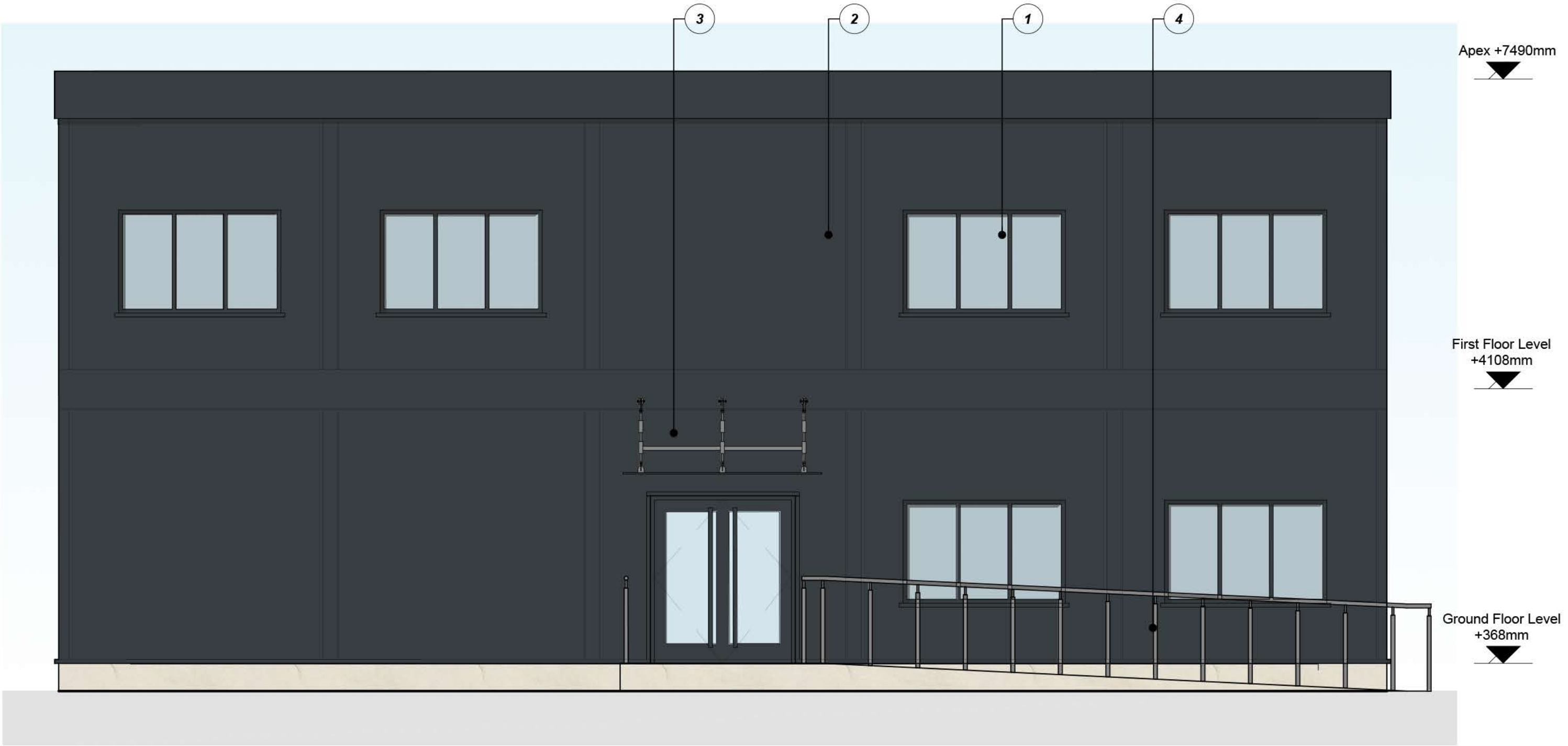
Amenity Building South Elevation Scale 1:50
