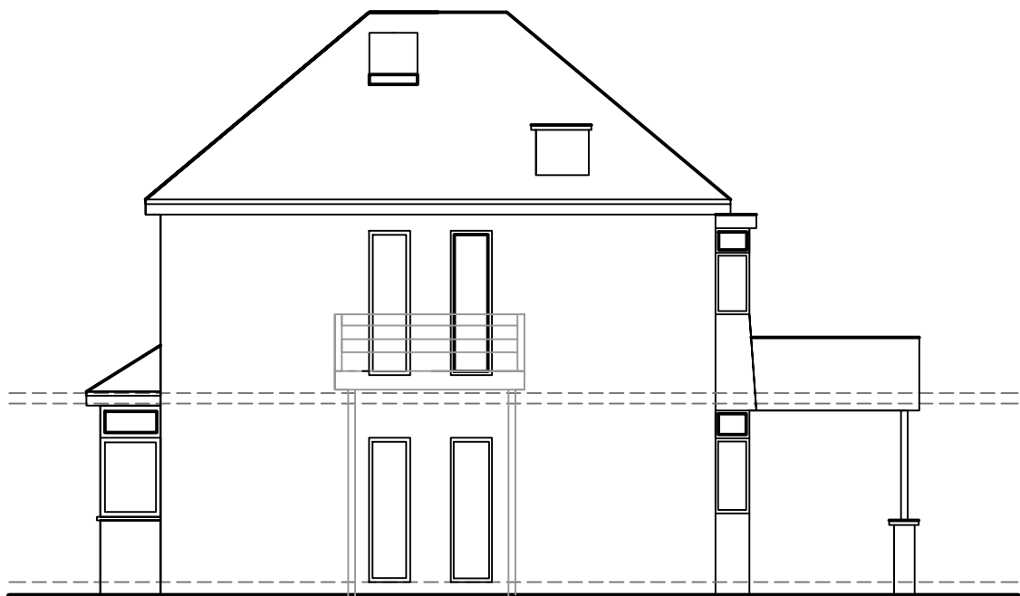
EXISTING SIDE ELEVATION 1:100
