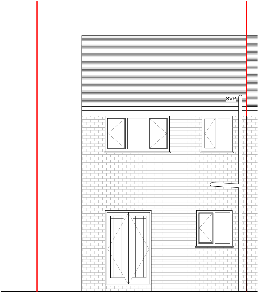
Existing Rear Elevation 1 : 50
