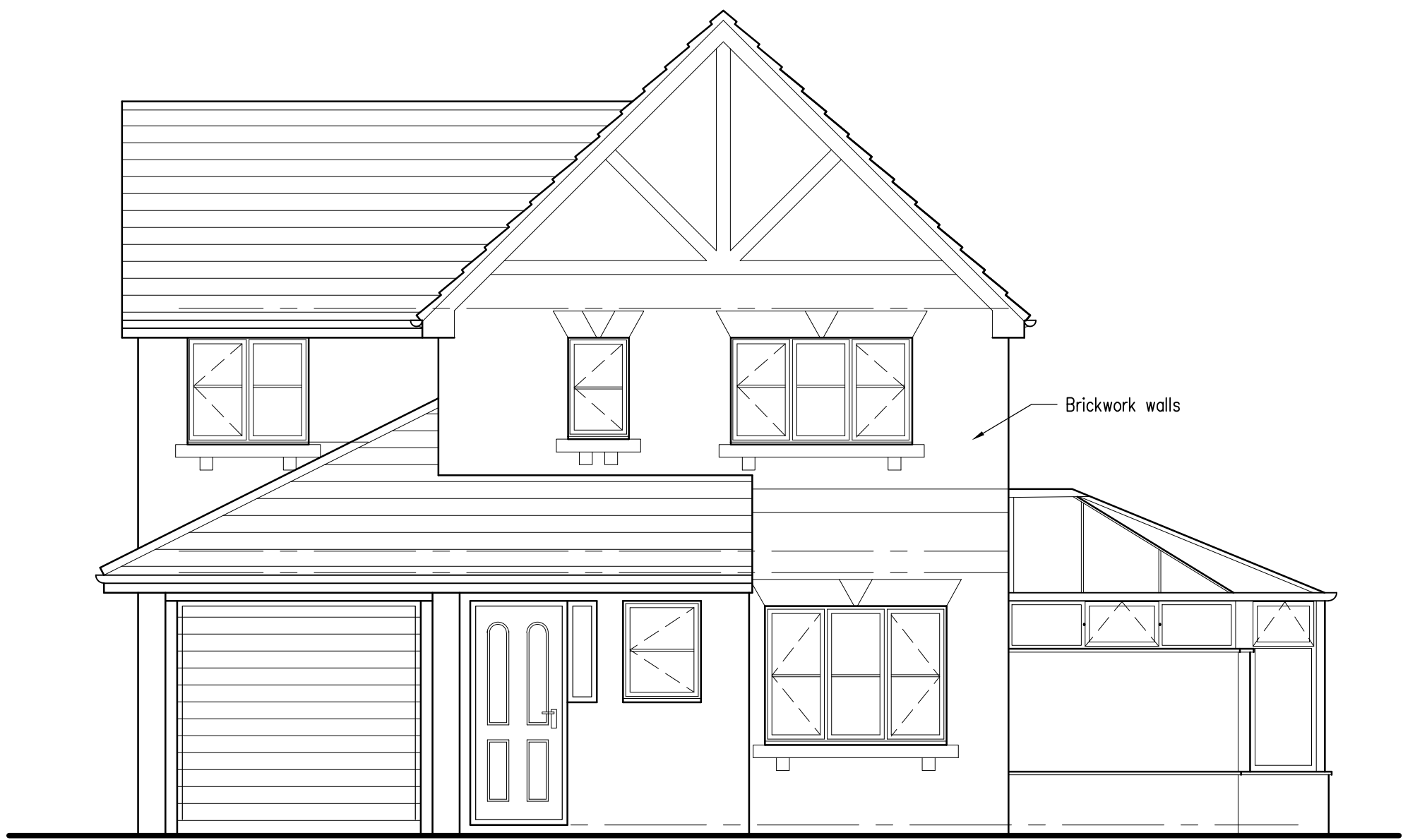
EXISTING FRONT ELEVATION
