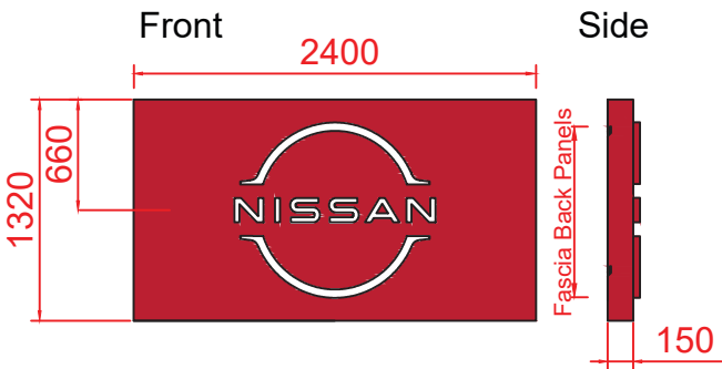
Sign D: NEXT Boutique Red Tablet Size 4 Logo Illumination: Internally Illuminated with White LEDs Material: Internal Aluminium Frame 4mm ACM - Nissan Red NVR-01, RAL3001, PMS200 Scale 1:50 @ A3
