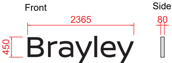
Sign C1, C2: Dealer Name Size 4 Individual 3D letters Face Illumination: Internally Illuminated with white LEDs Material: 1mm Hairline S/S Returns 4mm Black/White Acrylic Front Face Scale 1:50 @ A3
