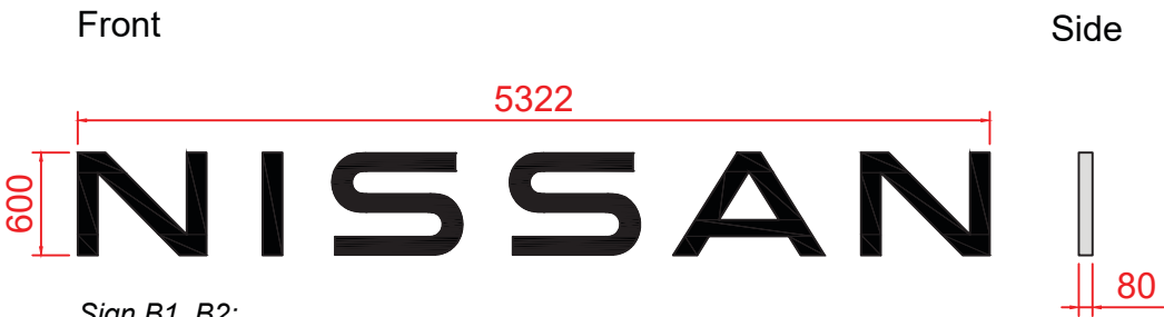
Sign B1, B2: Nissan Wordmark Size 4 Individual 3D letters Face Illumination: Internally Illuminated with white LEDs Material: 1mm Hairline S/S Returns 4mm Black/White Acrylic Front Face Scale 1:50 @ A3
