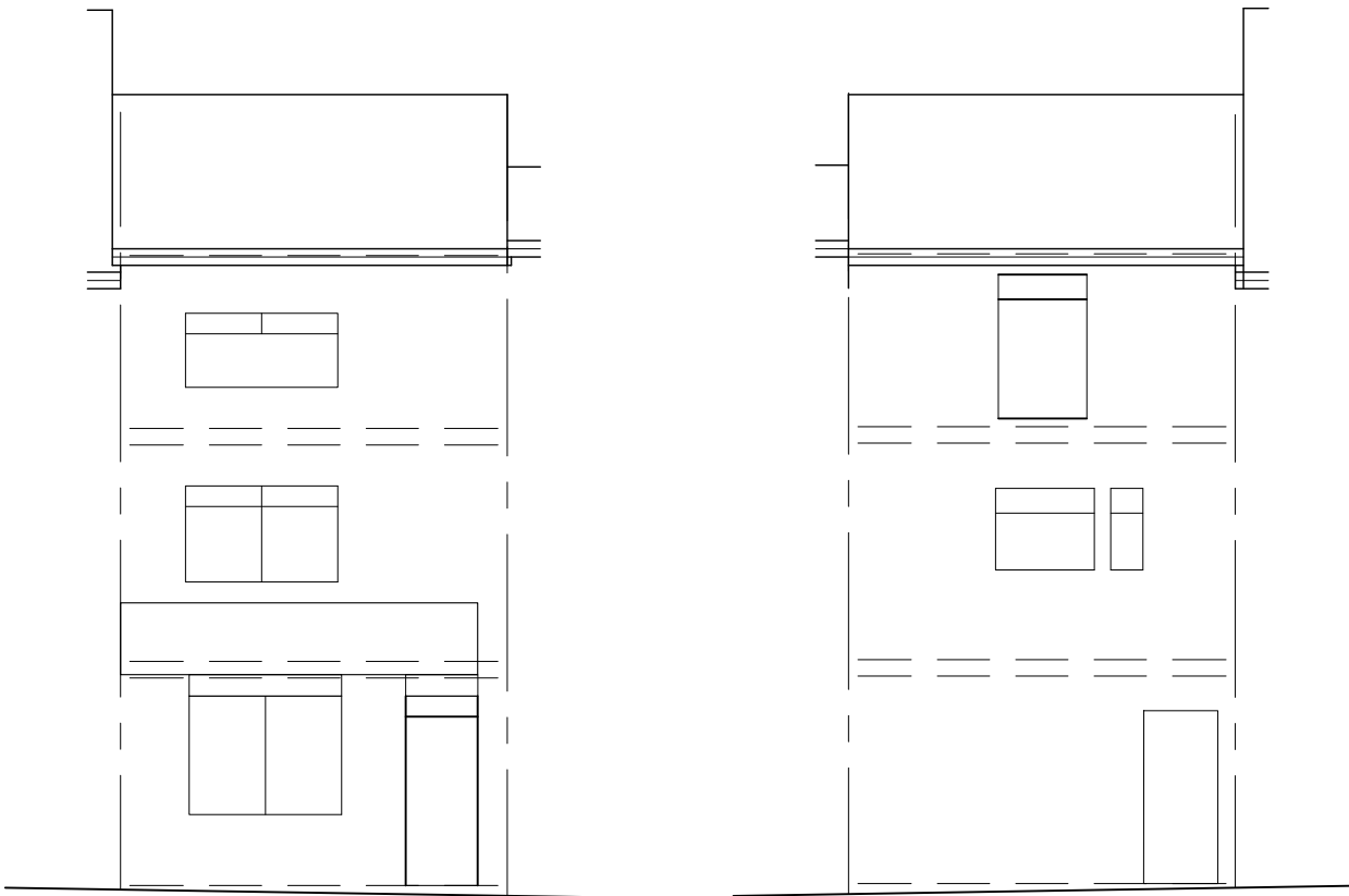
FRONT ELEVATION (EXISTING)
